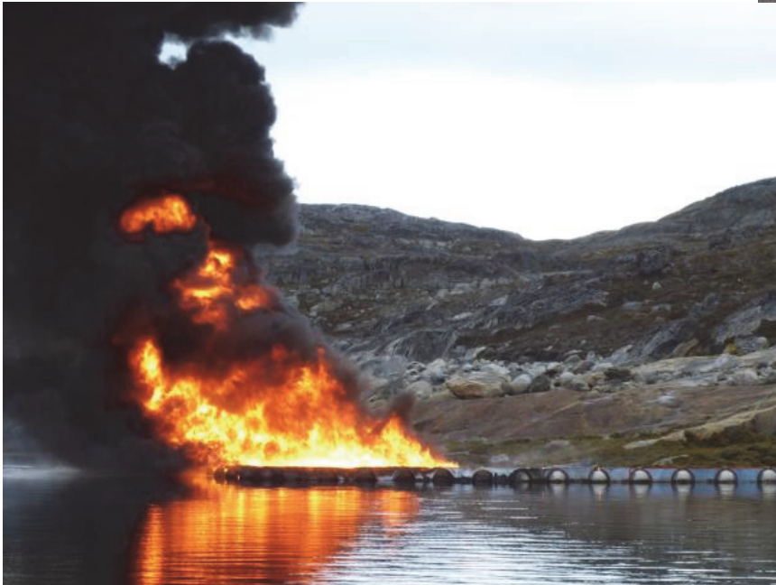
Shoreline experimental in situ burning
