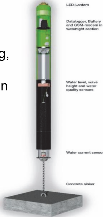
Schematic diagram of the SmartBuoy concept
