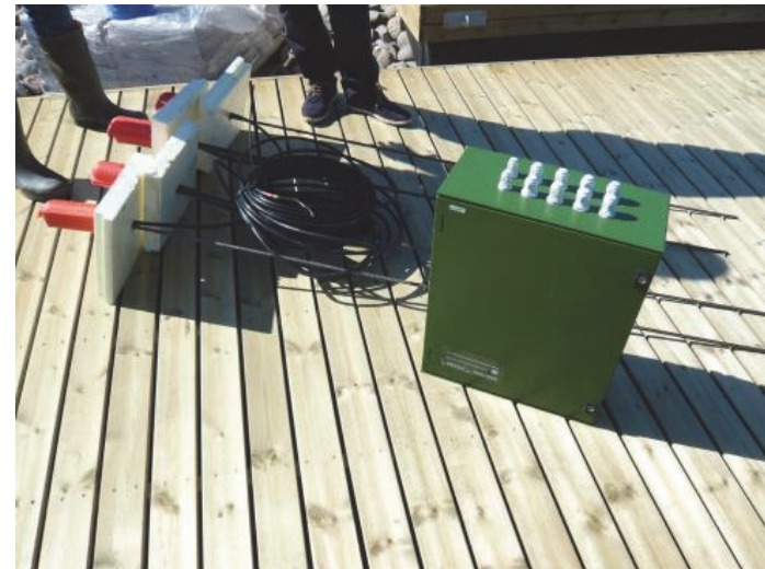
Electrodes for electrokinetic treatment of sediment
