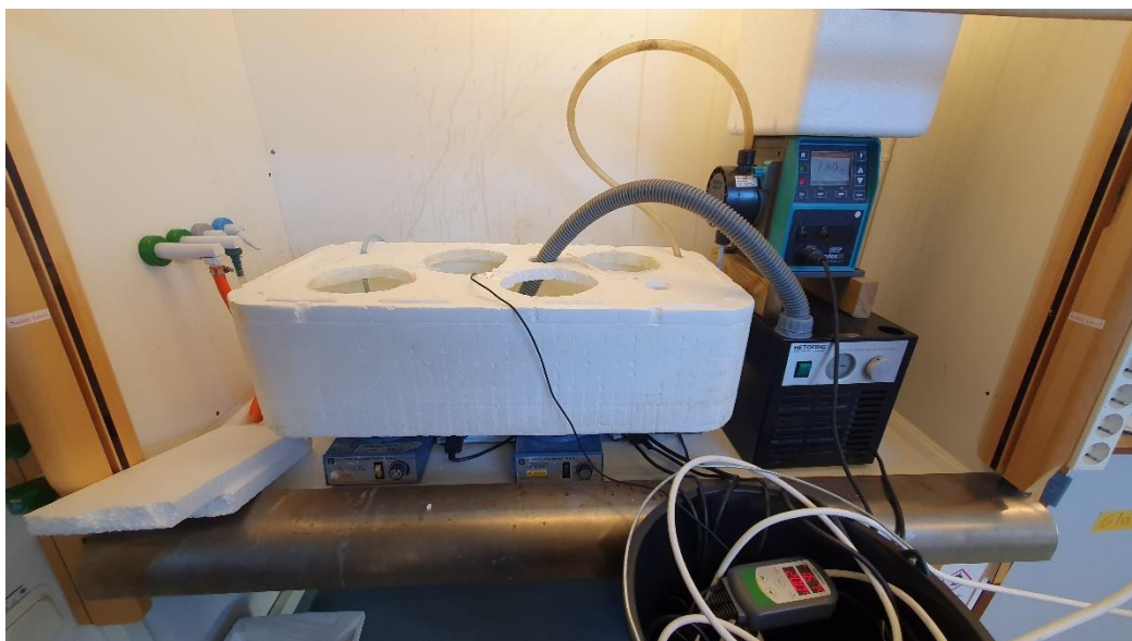
Figure 20. The water bath which has a cooling apparatus controlled by a temperature sensor.
