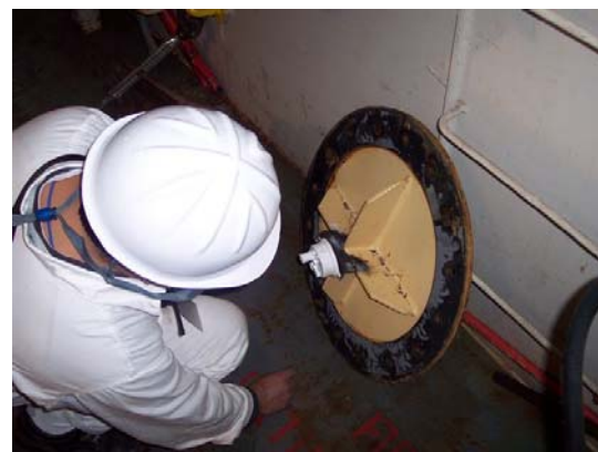
Picture 3.4.2 Cement hole cover in pontoon and mounting of Rh_2
