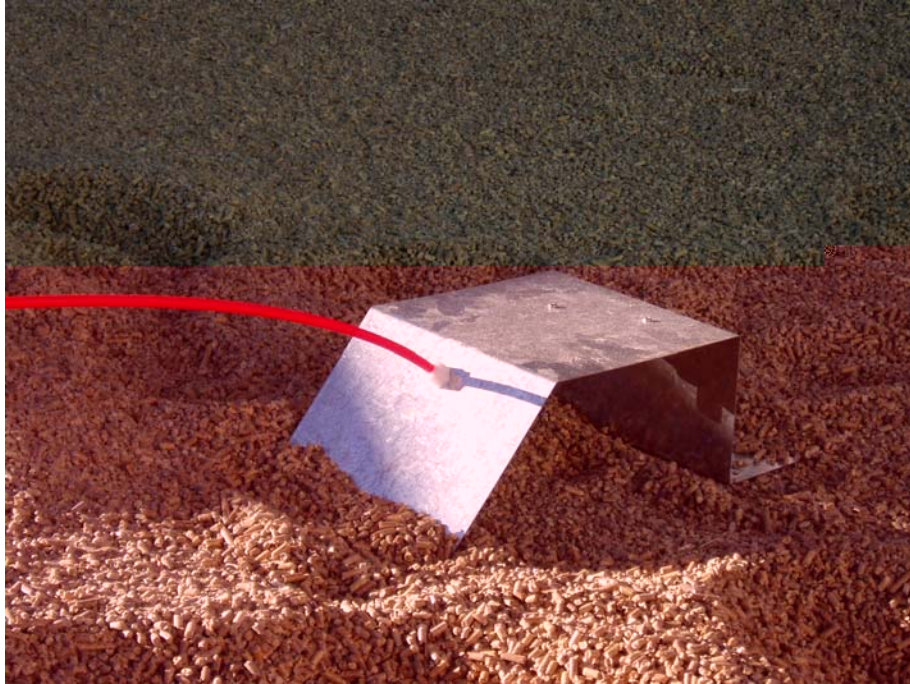
Picture 3.4.1 Bracket for Rh_1 data logger combined with support for Sampling Head G_1
