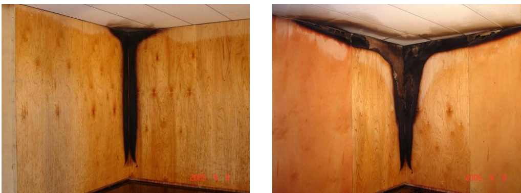
Figure 13 Illustrative results from two fire tests, where the nozzle used in the photo on the left hand side had wall wetting capabilities superior of the nozzle used in the photo on the right hand side. The fire source consisted of a 100 kW propane gas burner positioned close to the corner walls (not shown in the photos).
