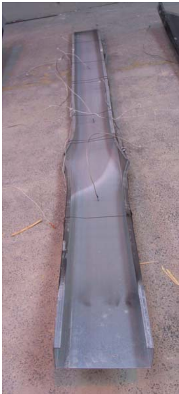
Figure 4-24: C-sections specimens after the fire tests (C 250)
