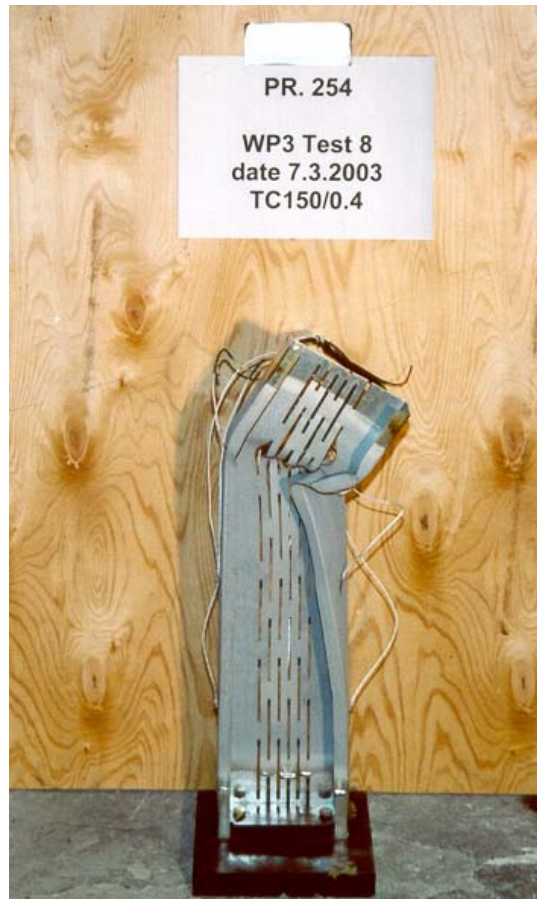
Figure 4-9: Test specimen 8 after fire test
