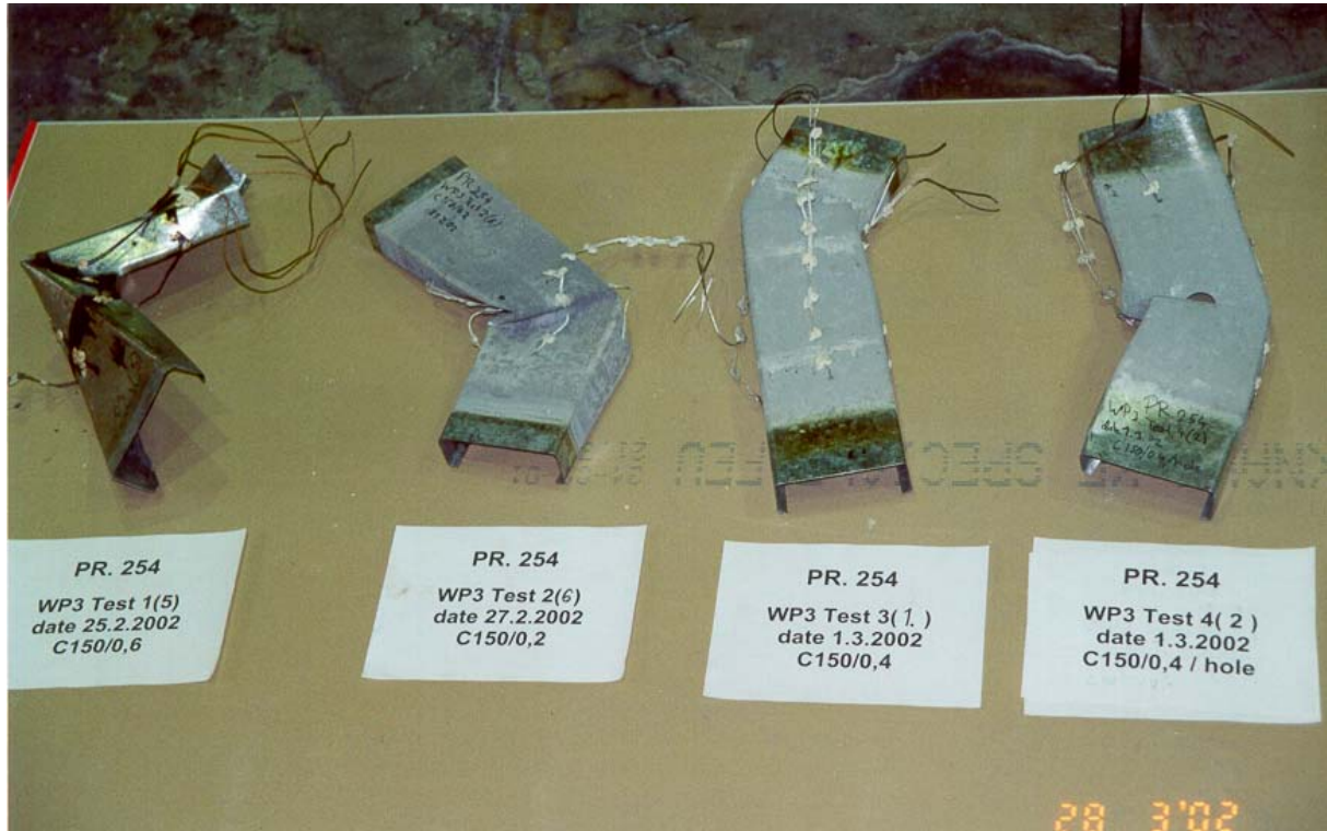
Figure 4-7: Test specimens 1–4 after the fire tests
