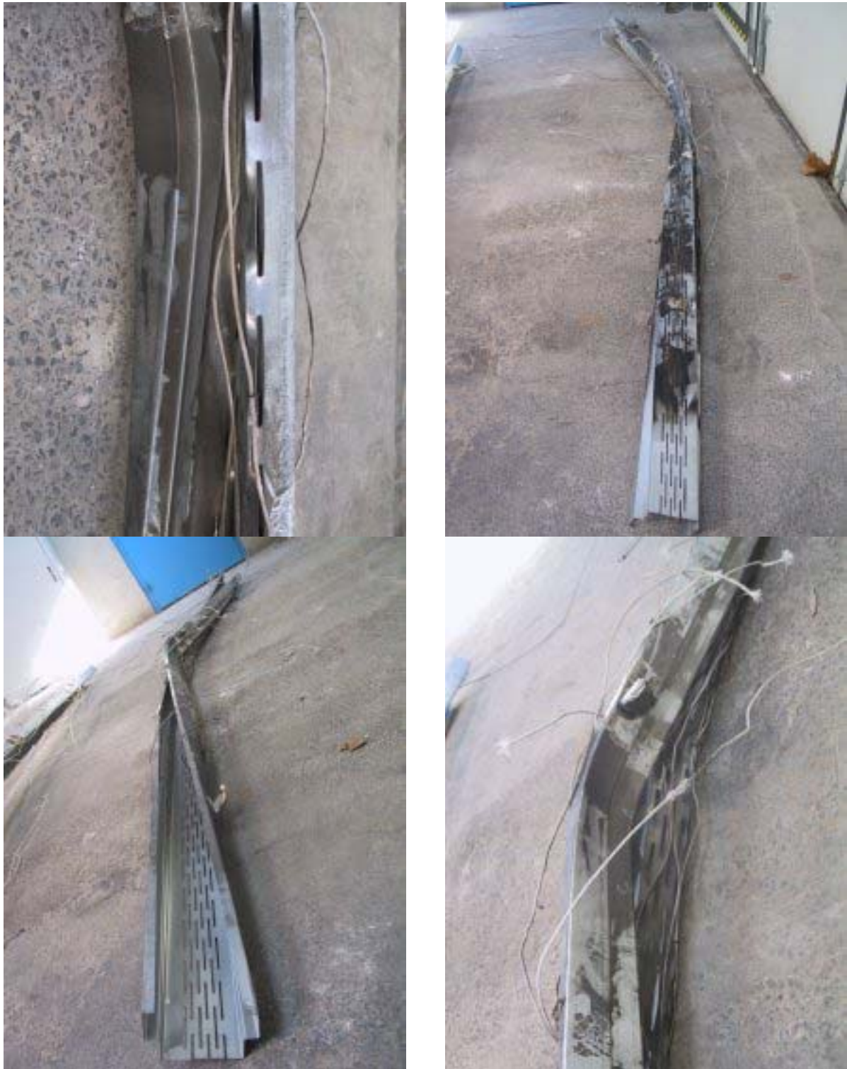
Figure 4-26: AWS-section specimen after the fire test
