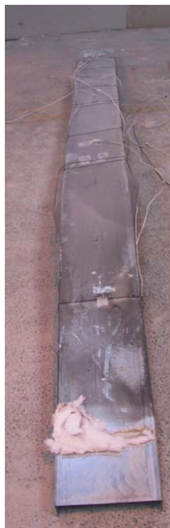
Figure 4-25: C-sections specimens after the fire tests (C 250)
