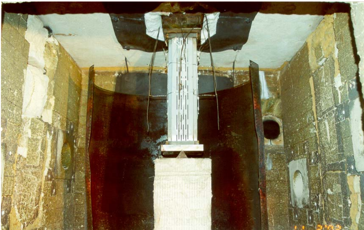
Figure 4-6: Mounting of the specimen (AWS-section)
