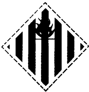
Division 4.1 Inflammable solids Symbol (flame): black Background: white with vertical red stripes
