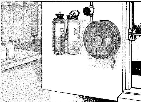
Position fire extinguishers close to the exit and keep clear
