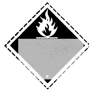
Division 4.3 Substances which, in contact with water, emit inflammable gases Symbol (flame): black or white Background: blue
