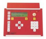
As an alternative to the PC the operator also has access to a control panel. The panel is easy to use thanks to a menu displayed on a screen, and provides the operator with complete control over all sirens, even when a map can't be dis
