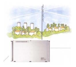
The master control unit is the heart of the system and is played on a specific stand, shielded against electromagnetic pulses (EMP), usually alongside other electronic equipment. The master control unit handles all information to and from the sirens and the PC stores all information about the system.
