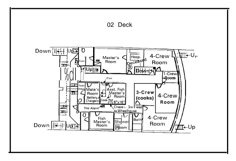
Figure 5 — Enlarged plan view of the 02 deck
