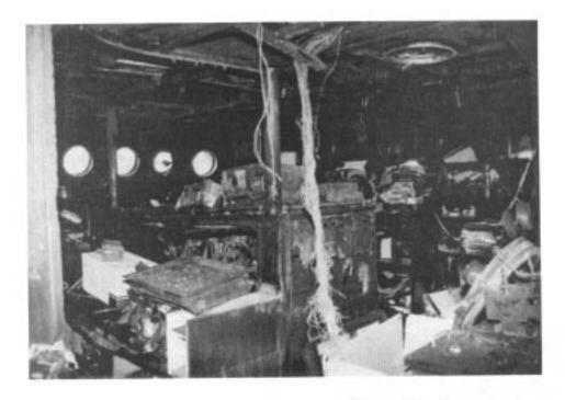
Figure 8 — Fire-damaged wheelhouse, revealing overhead construction (courtesy NFPA, Quincy, Massachusetts)
