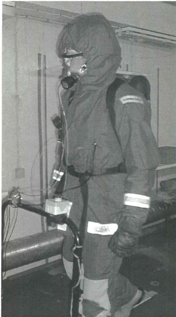
Figure 2. A fully equipped fire fighter walking on a treadmill in the heat (45 °C)
