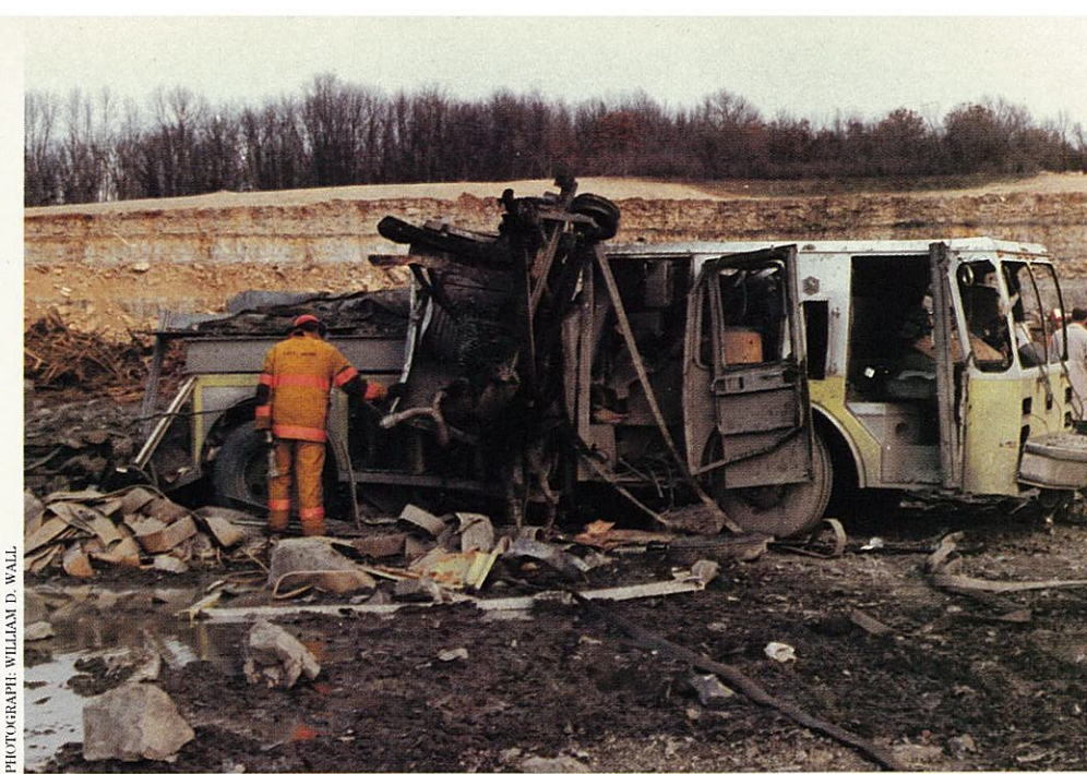
PHOTOGRAPH BY WILLIAM D. WALL The force of the blasts was so powerful that it blew the chassis of a light trailer into the side of Pumper 30 and almost through the other side of the engine.
