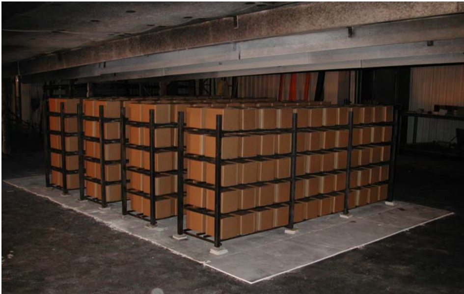
Figure 2.4 Experimental set-up: racks with cardboard boxes under a sloping ceiling (1:16) with beams (test 5.5).
