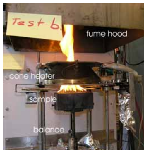
Figure 1-1: Sample compartment of the cone calorimeter.
