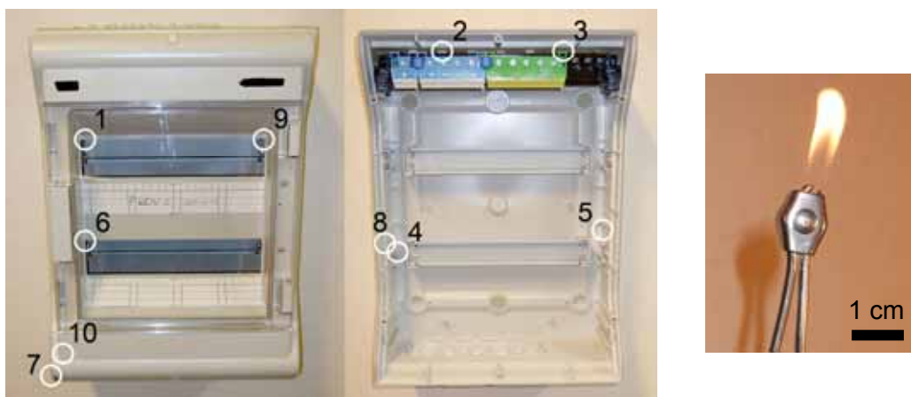
Figure 1-34: Left: Positions of flame application or placement of methamine pills for the full scale test. The burner was introduced through the flexible cable inlet to reach positions 1, 5, 6, 8 and 9 from the inside of the enclosure. Right: Burner outlet with the small premixed flame.
