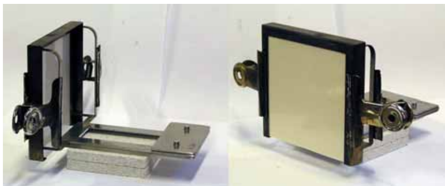
Figure 1-28: Two views of the sample holder used for the vertical cone calorimeter experiments.
