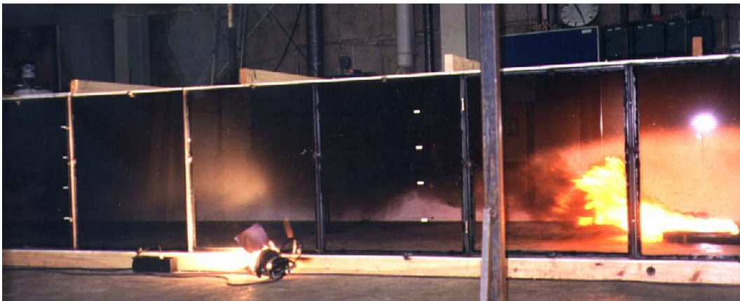
Figure 2 A photo of the model scale test tunnel. The fire source consisted of a Kerosine fuel.
