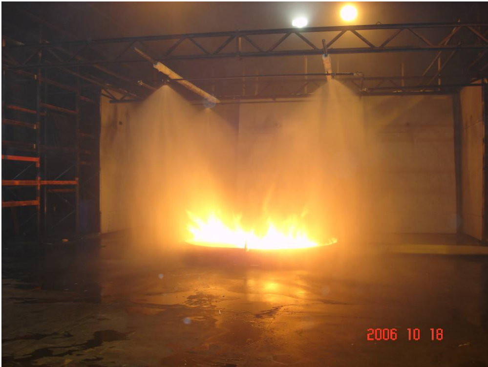
Photo 5 Test 1: The fire was suppressed almost immediately.
