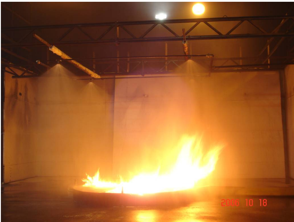
Photo 8 Test 2: This fire controlled by the system, at a discharge density of 5,0 mm/min.
