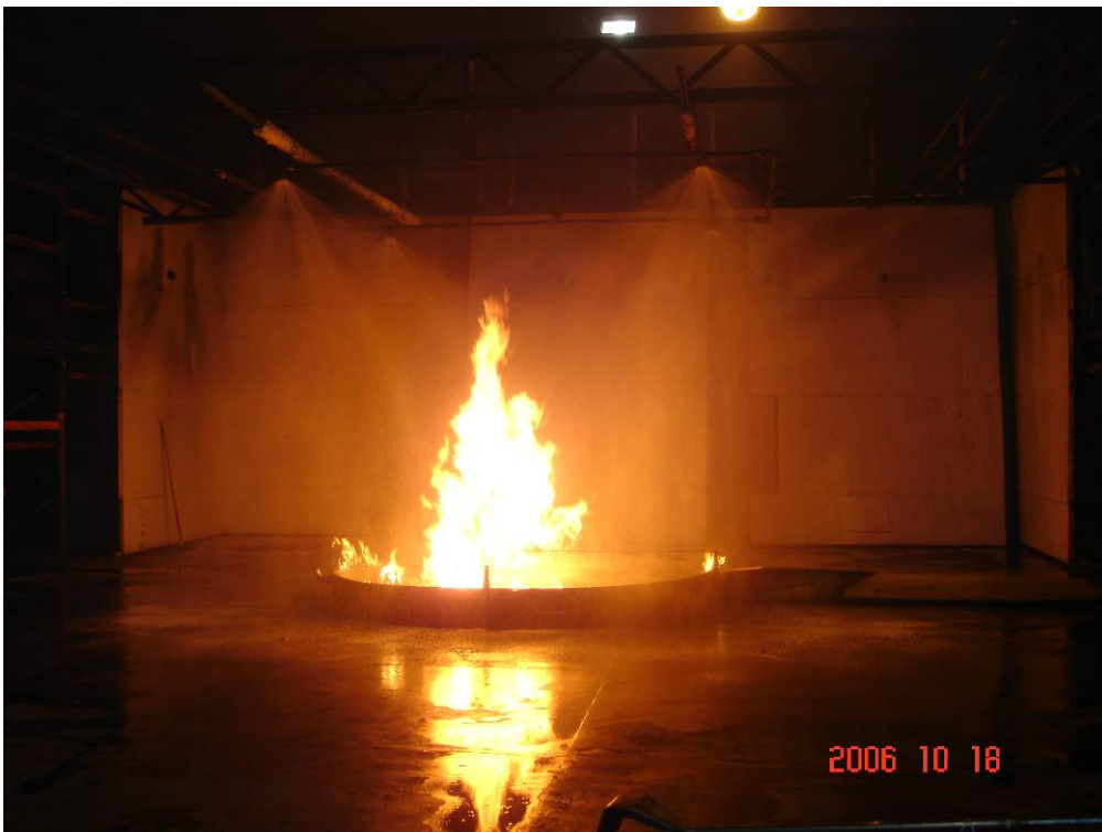
Photo 10 The use of foam in Test 4. A layer of foam has started to build across the fuel surface.
