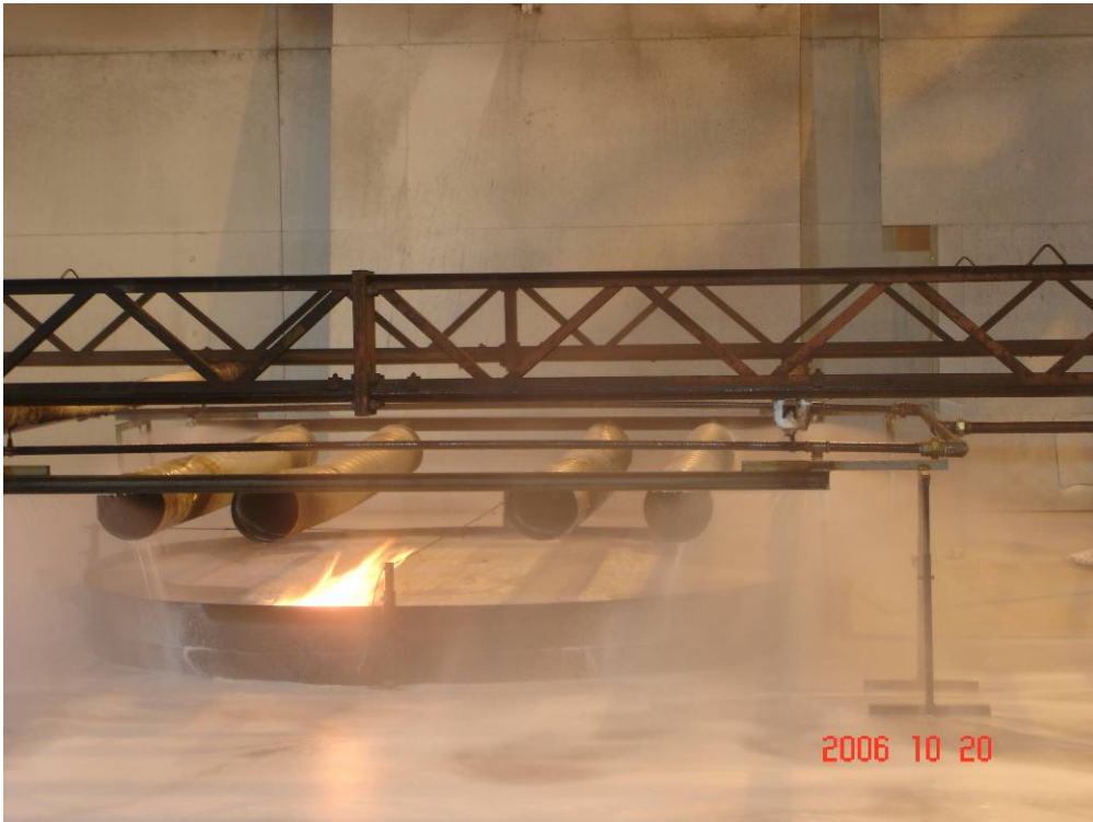
Photo 21 Test 13: Moments before full fire extinguishment. The surface is almost completely covered by a layer of foam.
