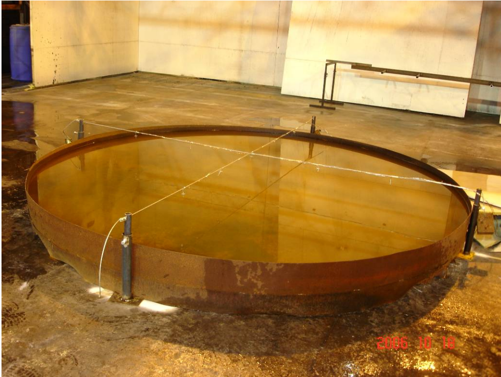
Photo 1 The 3,0 m diameter (7,07 m 2 ) fire tray, with the steel wires with attached thermocouples above the fuel surface.
