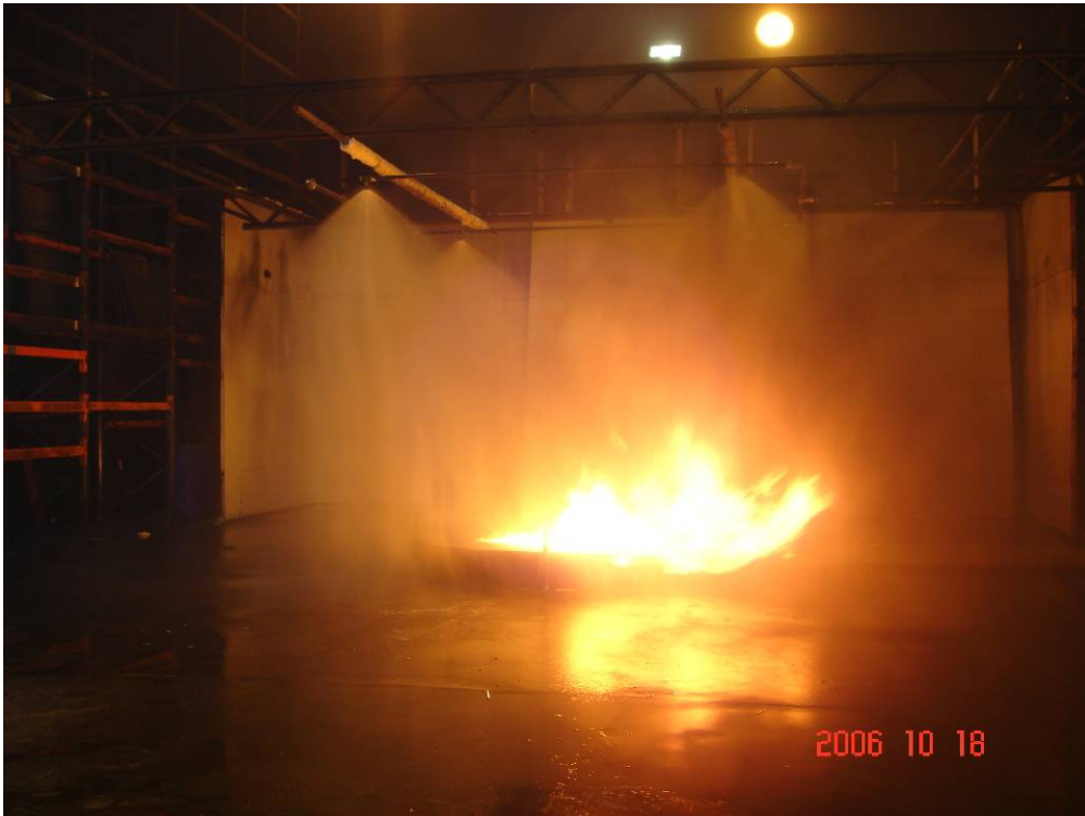
Photo 7 Test 1: The fire size increased after approximately eight minutes, but was still kept down by the system.
