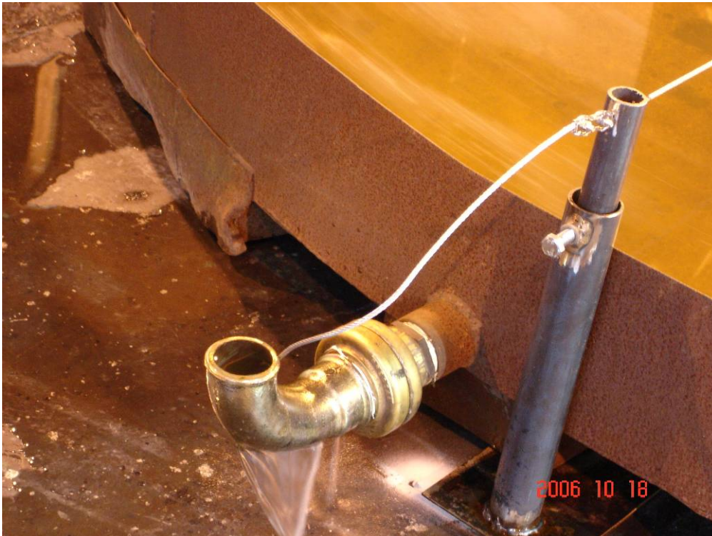
Photo 2 The overflow device that kept the rim height constant.
