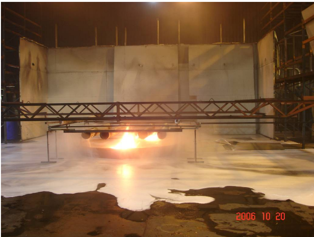
Photo 20 Test 13: The foam that did not enter the fire tray spread across the floor of the fire test hall.
