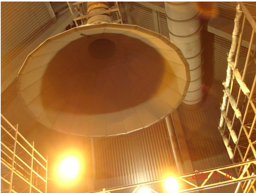
Photo 4 The Industry Calorimeter that was used to measure the convective Heat Release Rate.
