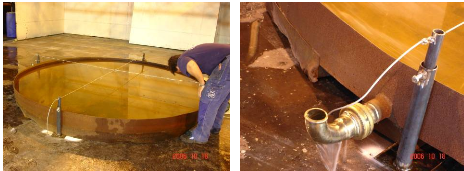
Figure 5 The fire tray used in the tests with the wire thermocouples positioned above the pool fire surface. To the right, the overflow device at the side of the fire tray that kept the level of fuel constant is shown.
