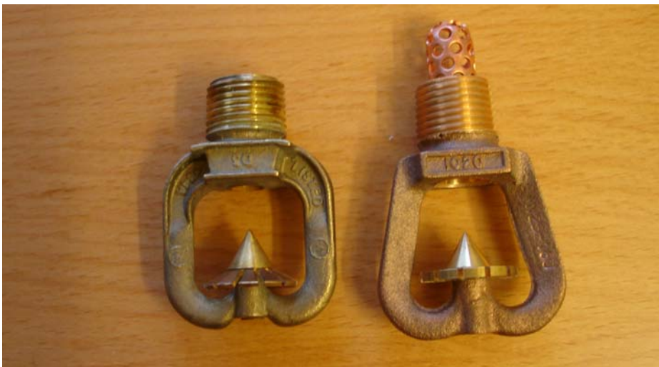
Figure 4 The type of nozzles used in the tests, to the left a D3 Protectospray nozzle and to the right a Wormald MV nozzle.
