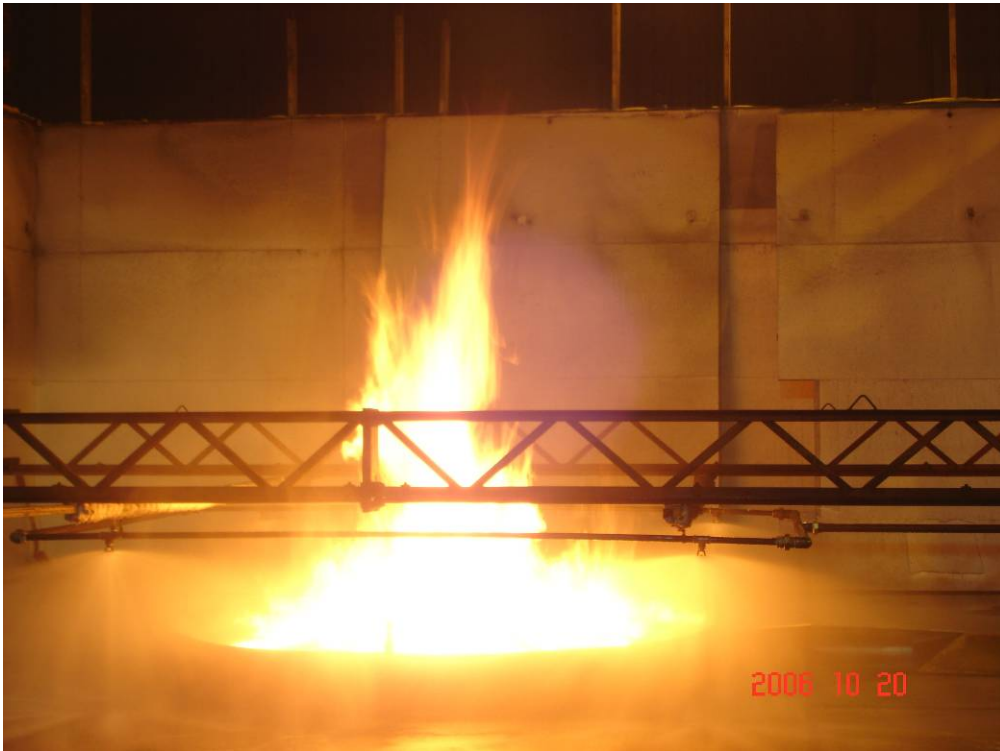
Photo 15 Test 11: When the water discharge density was increased to 10,0 mm/min, 'fire control' was achieved.
