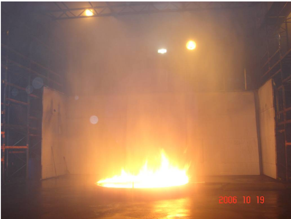
Photo 12 For Tests 7 – 9, the grid of nozzles was installed 6,5 m above the fire. In Test 7 (pictured), the water discharge density of 7,5 mm/min provided fire suppression and eventually fire extinguishment (see Photo 13).
