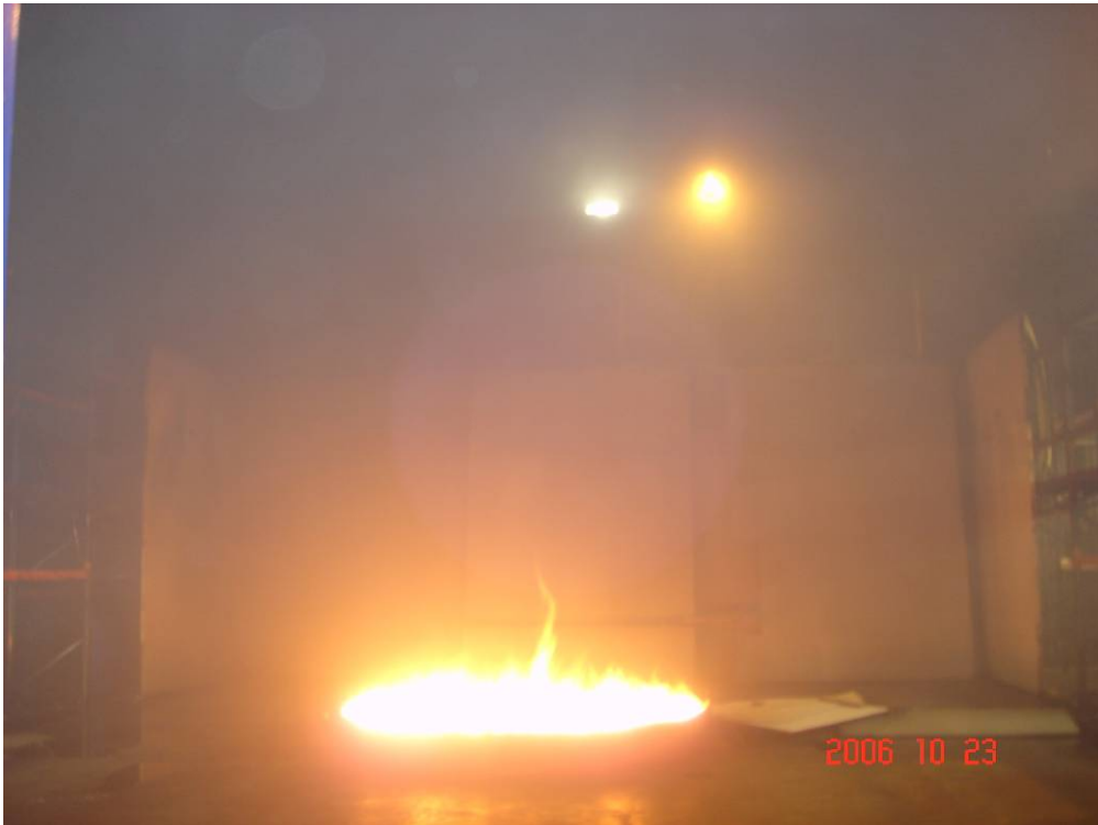
Photo 23 Test 14: The fire size is reduced, although flames are covering the whole of the surface.
