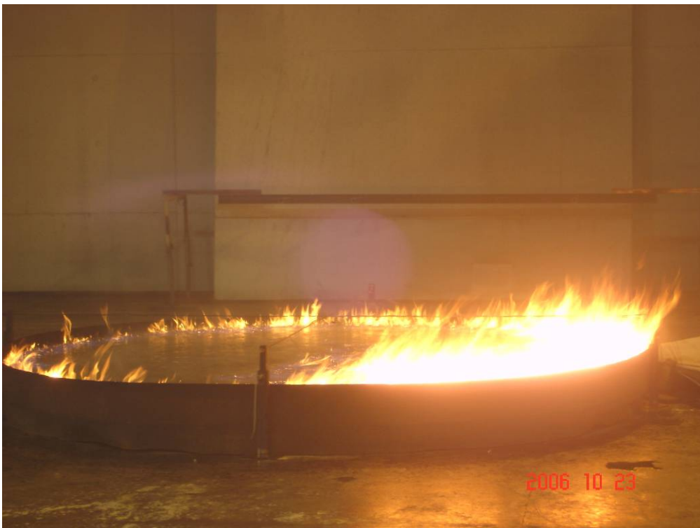
Photo 24 Test 14: Small flames, primarily around the perimeter of the fire tray.
