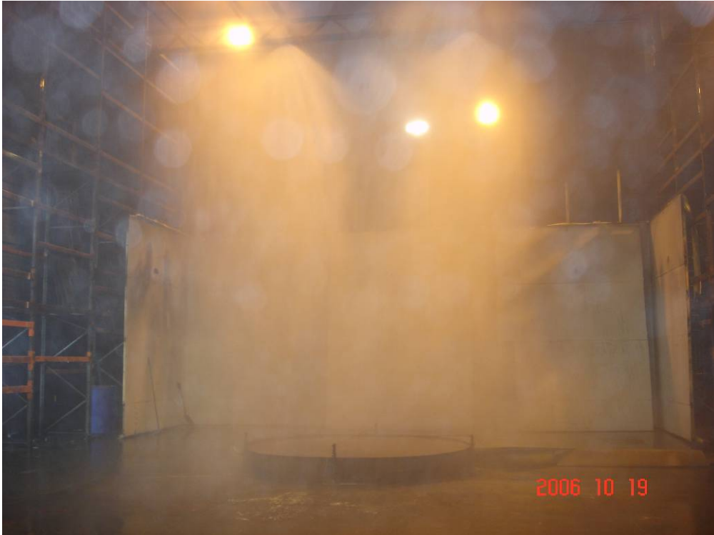
Photo 13 Test 7: Fire extinguishment at 02:10 [min:sec].
