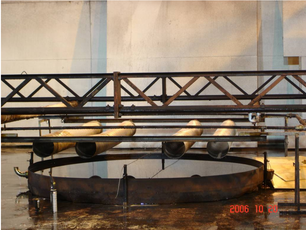
Photo 17 The four \text{\O}=250 mm steel pipes that was used to obstruct the pool fire surface in Tests 12 and 13, respectively.
