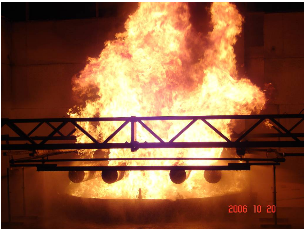
Photo 18 Test 12: Only a limited degree of fire control was achieved, as a large portion of the water spray from the nozzles were obscured by the steel pipes.
