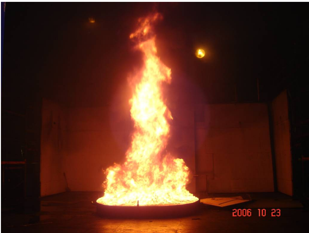
Photo 22 Test 14: The free-burn fire test, after approximately 03:30 [min:sec] after ignition, where the fire is at its peak.
