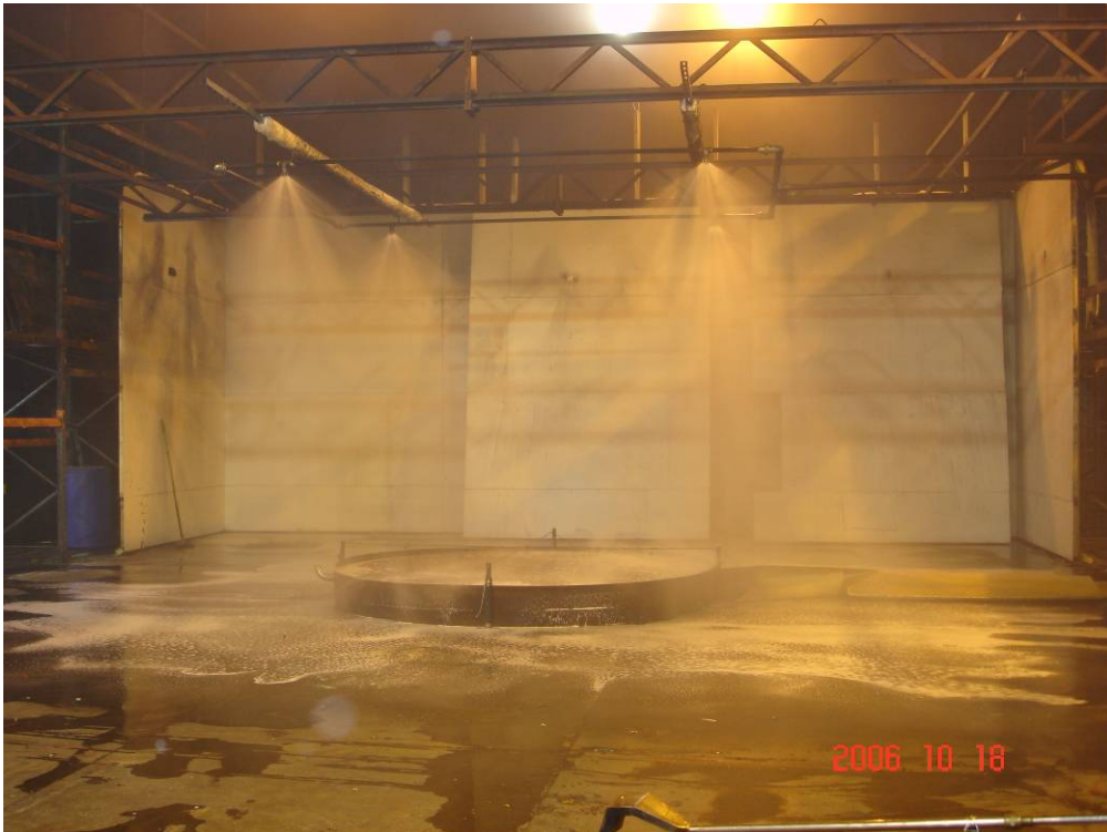
Photo 11 The final extinguishment in Test 4 occurred after only 20 seconds.
