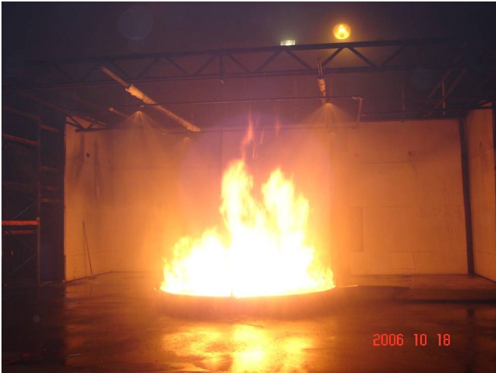
Photo 9 The typical 'limited fire control' scenario that was achieved by a discharge density of 3,5 mm/min in Test 3.
