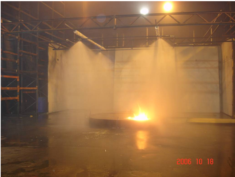
Photo 6 Test 1: During several minutes, the fire was virtually extinguished but continued to burn around the perimeter of the fire tray.
