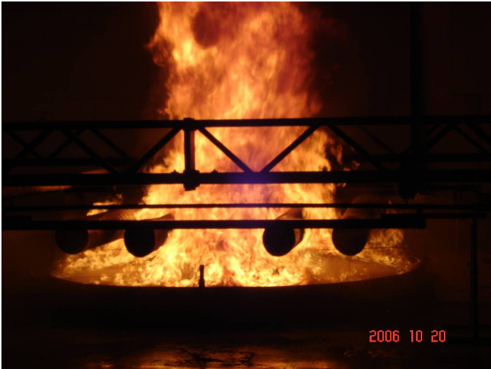
Photo 19 Test 13: An AFFF foam additive was used and the fire size was gradually reduced as the foam spread across the pool fire surface.
