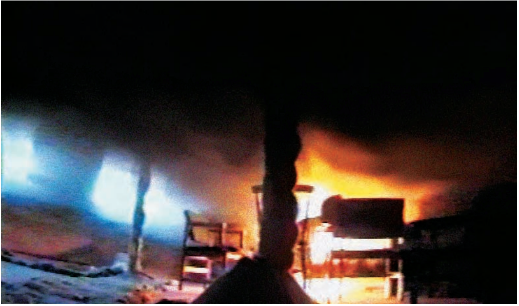
Figure 81 (above). The fire is about to spontaneously go out in a closed room. The smoke gases sink down above the seat of the fire. The only clear visibility is at floor level.
