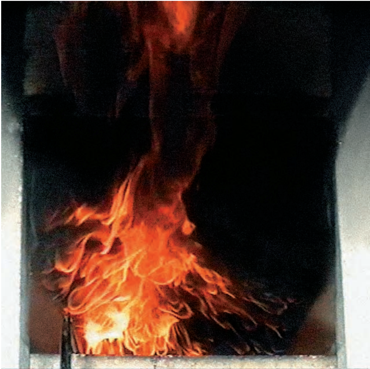
Figure 33. Flames on the under side of a smoke gas layer.
