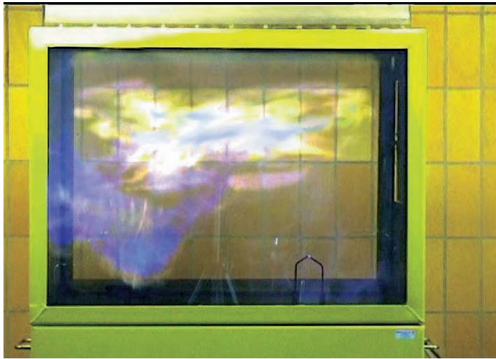
Figure 35. Premixed flames spread in an aquarium. An aquarium is used to demonstrate the flammability ranges for different gases. The most common combination used is liquefied petroleum gas (LPG) and air.
