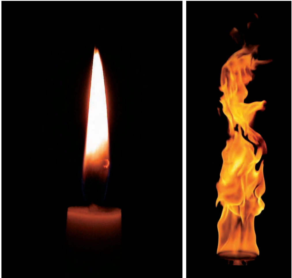
Figure 32. Laminar diffusion flame on the left. Turbulent diffusion flame on the right.
