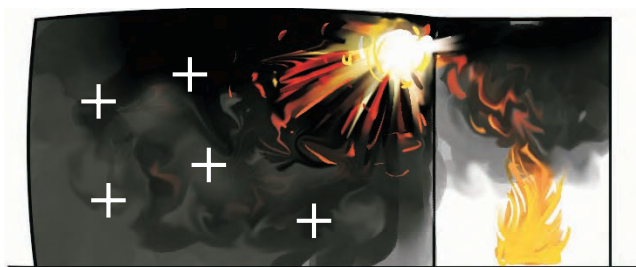
Figure 114. The smoke gases have leaked into the adjacent room and are ignited by a shooting flame.
