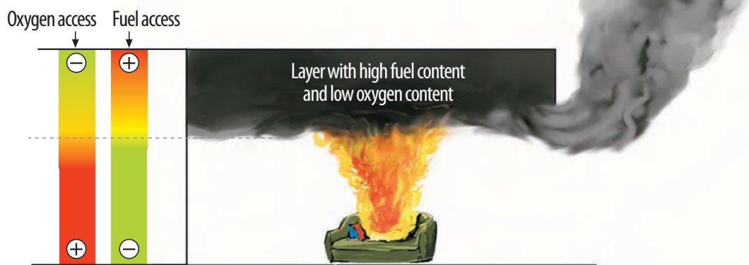
Figure 34. A high concentration of fuel high up will gradually cause the flames to reach the under side of the smoke gas layer.
