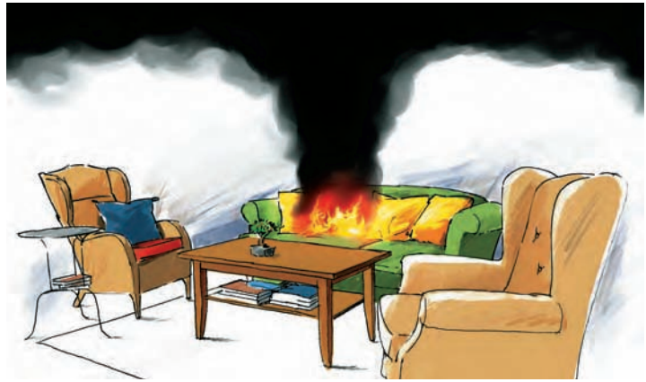
Figure 22. Smoke gases start to accumulate under the ceiling. But the atmosphere in the lower part of the room is still fine for a person to remain there for a short period of time.
