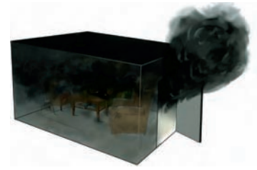
Figure 91. Air flows in and smoke gases escape.
