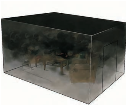
Figure 86. The smoke gases auto-ignite when they come into contact with air.
