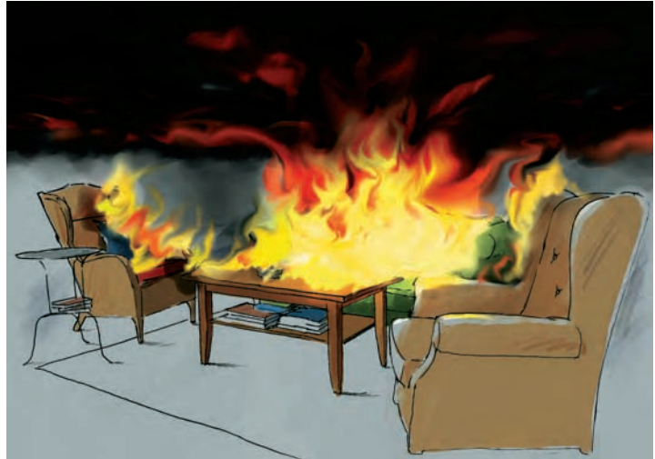
Figure 59. The fire has spread to other objects in the room. Soon the whole room will be involved.
