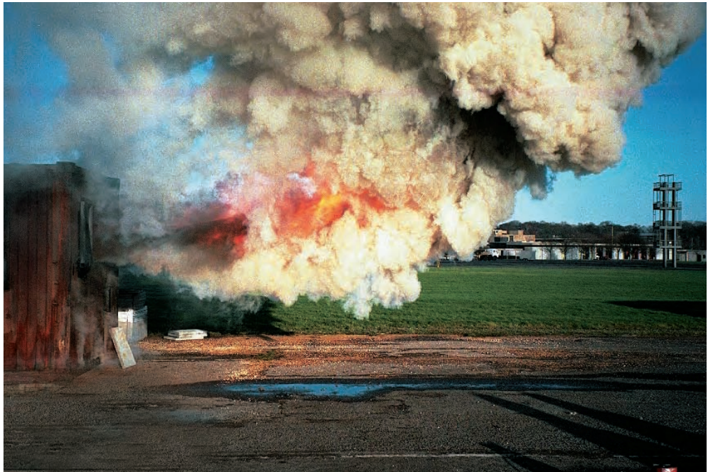
Figure 68. White smoke gases are definitely not harmless. In this case, the fuel is some type of wooden boards fitted at ceiling level. The colour of the smoke gases is largely dependent on whether the fire is smouldering or burning with a flame.
