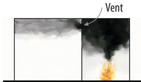
Figure 36. Smoke gases have leaked into an adjacent area. This is a fire scenario in which premixed flames can occur.
