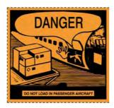
Name: Cargo Aircraft Only Cargo IMP Code: CAO Minimum dimensions: 120 x 110 mm Colour: Black on Orange
