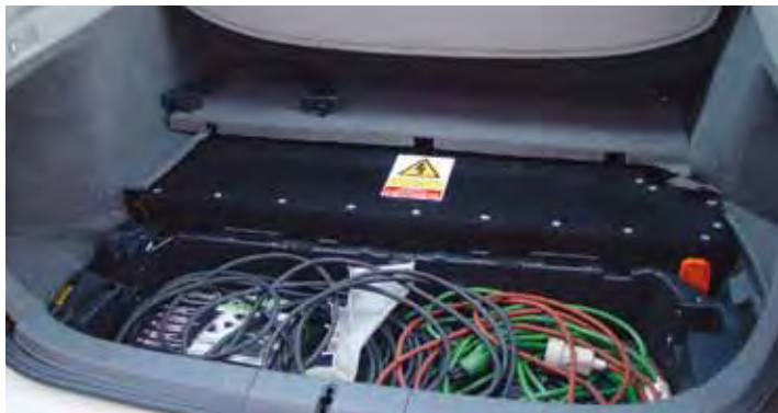
Many battery cells are coupled together to form a battery pack in the Prius
