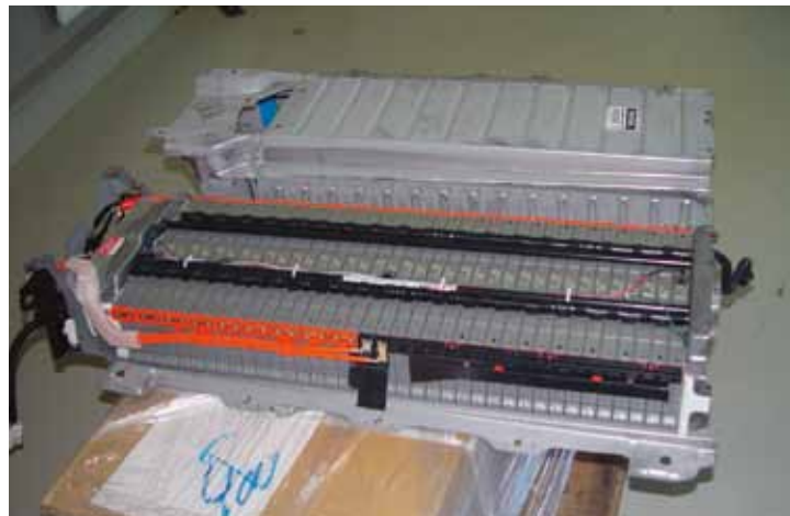
The protective covering removed from a metal hybrid battery pack. The battery is made up of many interconnected battery cells.
