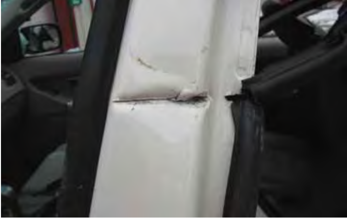
Cutting attempts on a B-pillar reinforced with boron steel.
