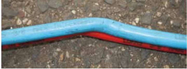
Poor hydraulic hose.
