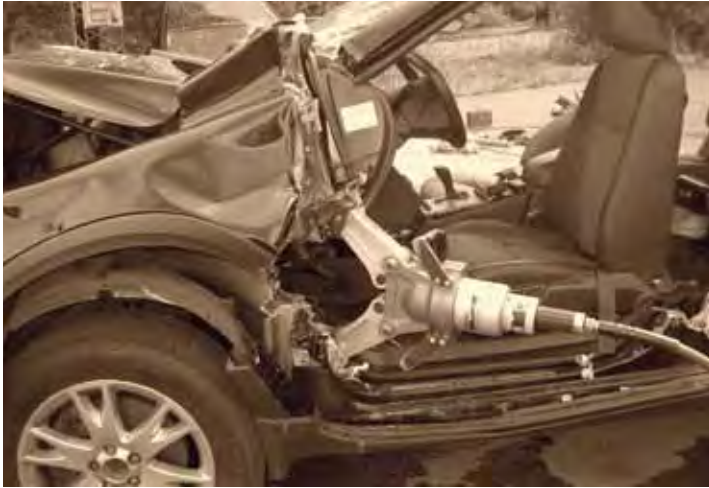
Lift carefully with the spreader.
