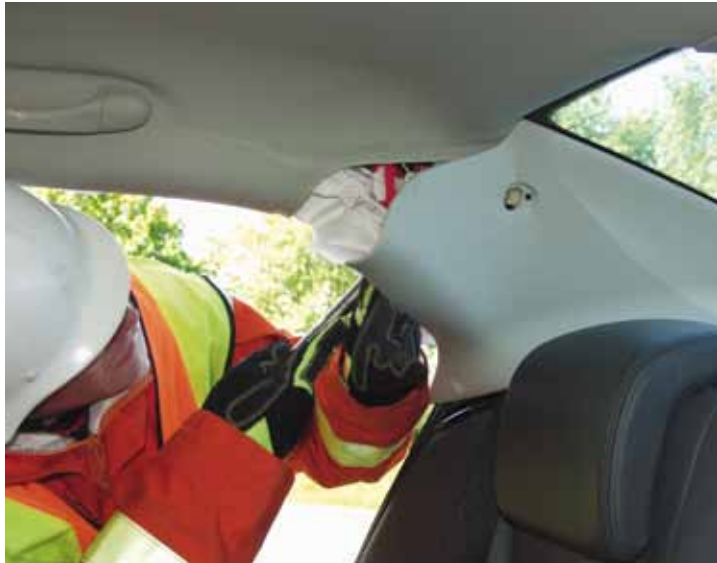
Break away the trim and look for where gas containers are located.
