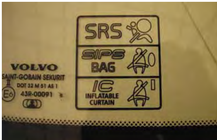
An airbag installation has to be identified, for example on a window, the dashboard or the steering wheel. The picture shows Volvo's identification of an airbag.
