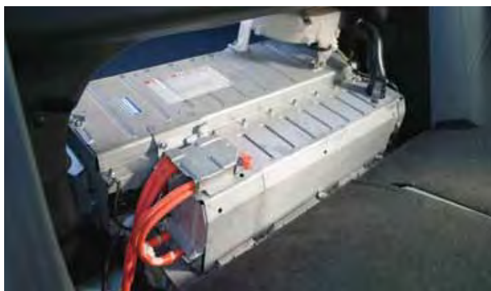
A battery pack in a hybrid car. Many battery cells are coupled together to form a battery pack.
