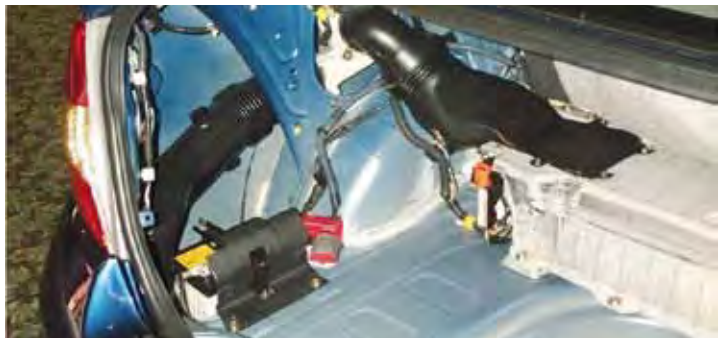
Boot of hybrid car. NOTE service switch and battery pack
