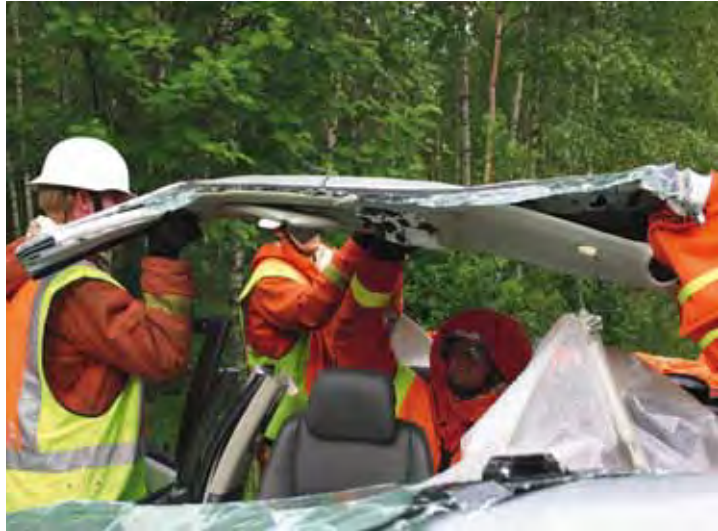
Lift off the roof.
