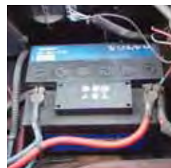
Closed lead-acid battery.
