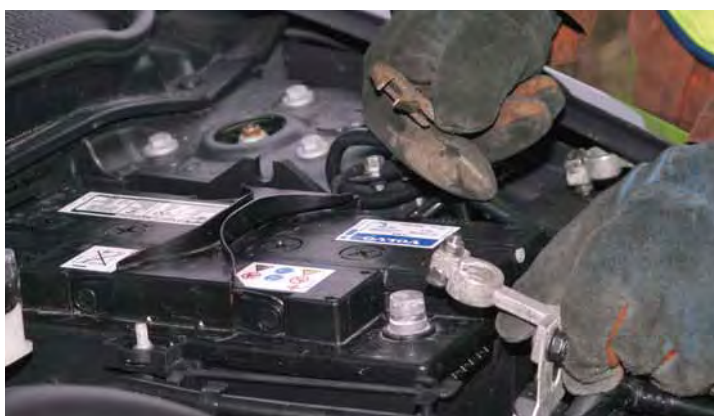
Disconnect the cables from the battery, negative cable first.
