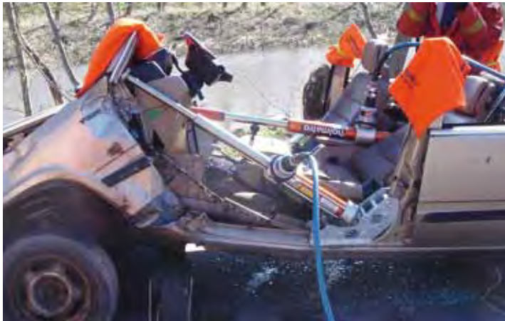
Press the dashboard forwards.
