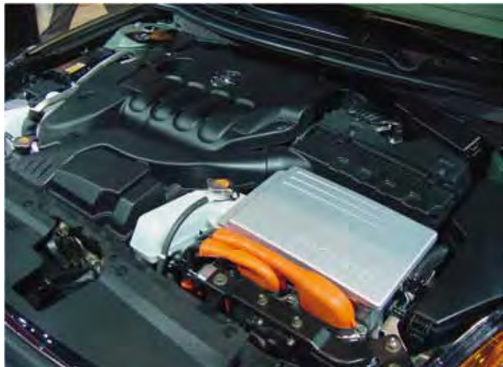
Engine compartment in a hybrid car. Orange = high voltage.
