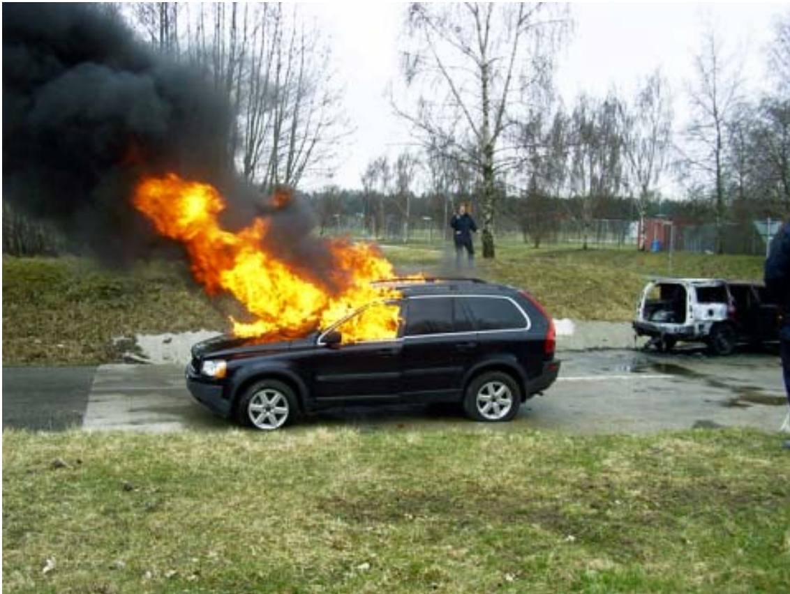
Picture 6.2-8: Full scale fire test, Volvo XC 90, Model 2003
