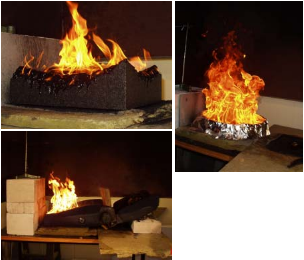
Picture 6.2-7: Fire tests in the third scale; top left: Neopolen; top right: polyurethane foam and heptane; bottom: Volvo 245 model car seat
