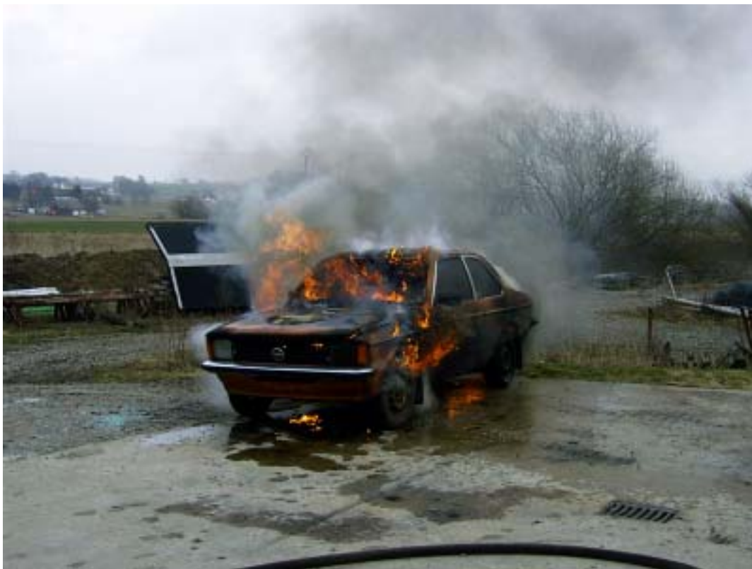
Picture 6.2-12: Full scale fire test, Opel Kadett, Model 1975
