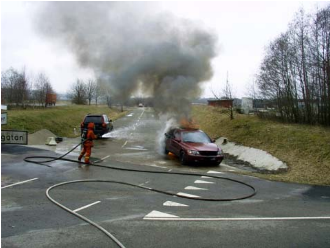
Picture 6.2-10: Full scale fire test, Volvo V70, Model 2004
