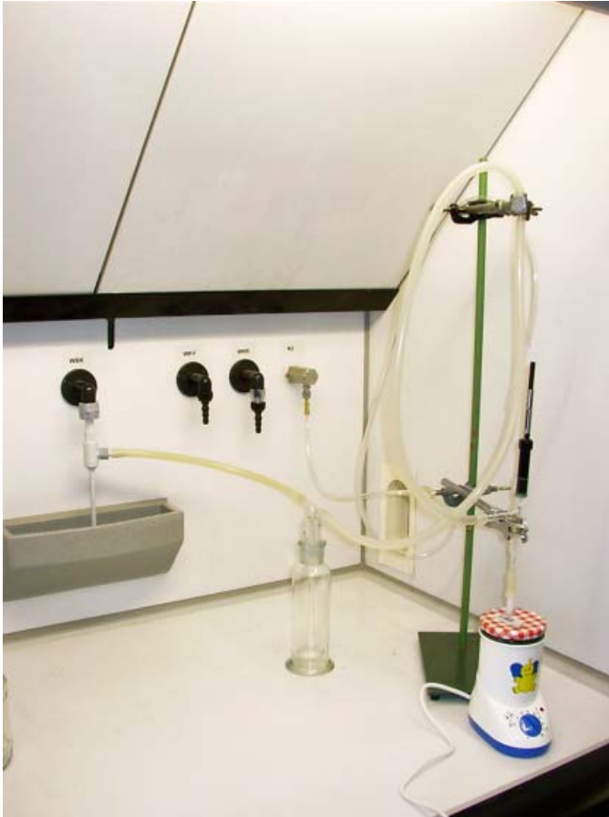
Picture 6.2-3: Overview of the extraction unit with water jet pump and safety washing bottle
