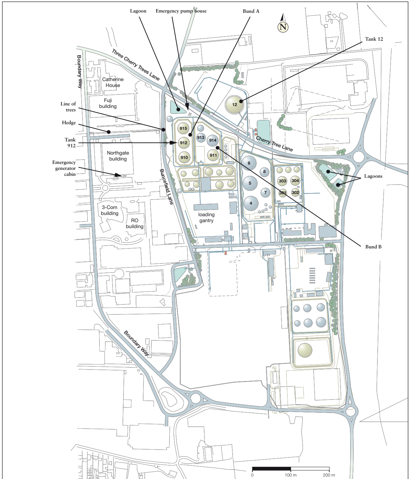
Figure 3 Pre-incident layout of Buncefield depot and immediate surroundings
