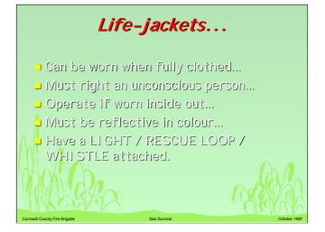
Explain the above. Emphasise that Crewsavers should be fitted with Snaplights but the new falcons are fitted with a water reactive light.
