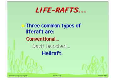
Three types of life-raft normally found. The Convential is a ships life-raft and found in containers around the vessel. the davit type is normally only found on fixed platforms.ie oil rigs and hangs inflated in a davit similar to a lifeboat.
