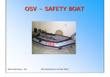
The boat is a 3.6m semi rigid inflatable with a 15hp outboard engine. With the boat will be :-throw lines, portable floodlight come torch, etc etc'
