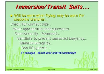
The suits will be demonstrated later. They are not Survival suits..purely for transit. They have no designed insulation/buoyancy.Make sure it fits and is not damaged. Wear firekit beneath for surface transit, Huggy Bear for helo. transit[because of air entrapment].Don correctly, vent . Beware of air migration and water ingress.Lifejacket.Operational procedures.
