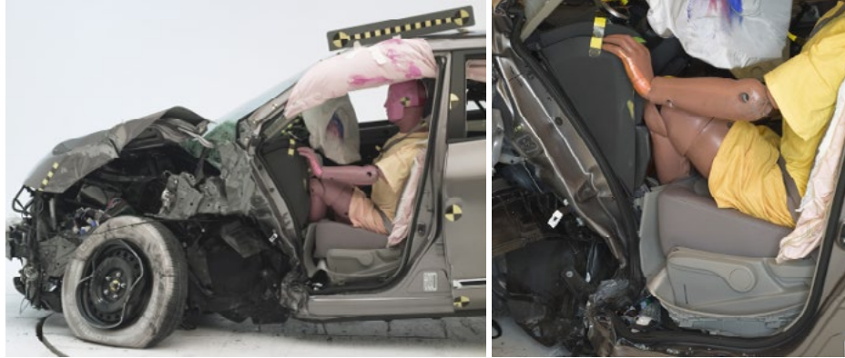
Figur 41. Small-overlap prov med 2014 Nissan Qashqai (CMF plattform)
