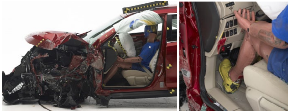
Figur 41. Small-overlap prov med 2014 Nissan Qashqai (CMF plattform)
