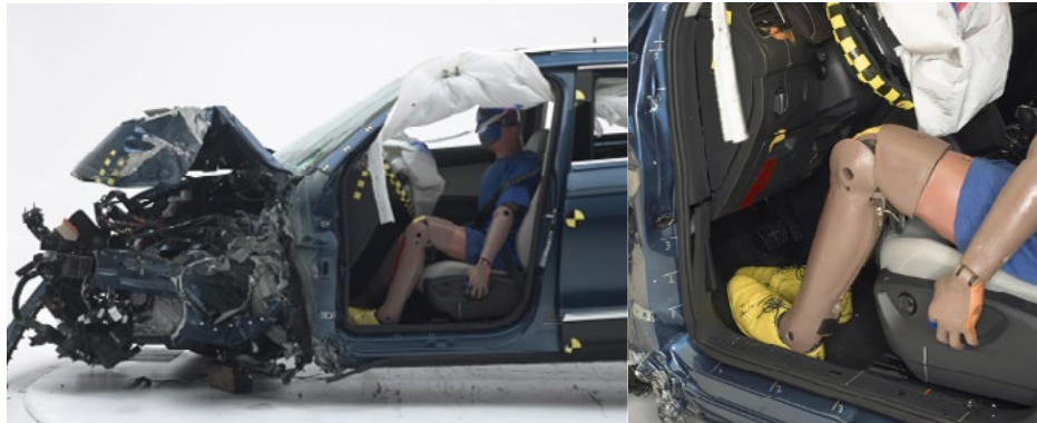
Figur 44. Small-overlap prov med 2018 Volkswagen Tiguan (MQB plattform)
