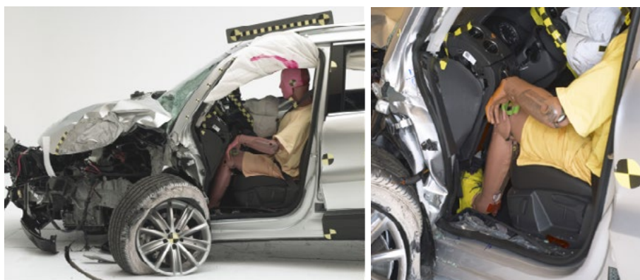
Figur 43. Small-overlap prov med 2013 Volkswagen Tiguan (PQ46 plattform)
