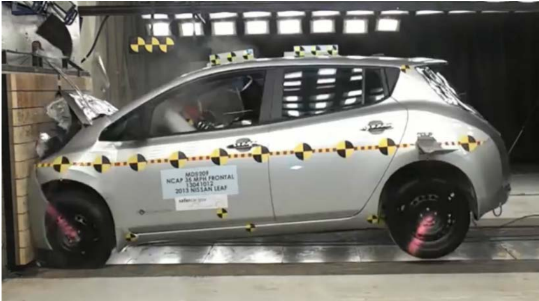
Figur 48 Frontal Crash – NHTSA NCAP Crash Test Video 2013 Nissan LEAF 5DR Hatchback (92)
