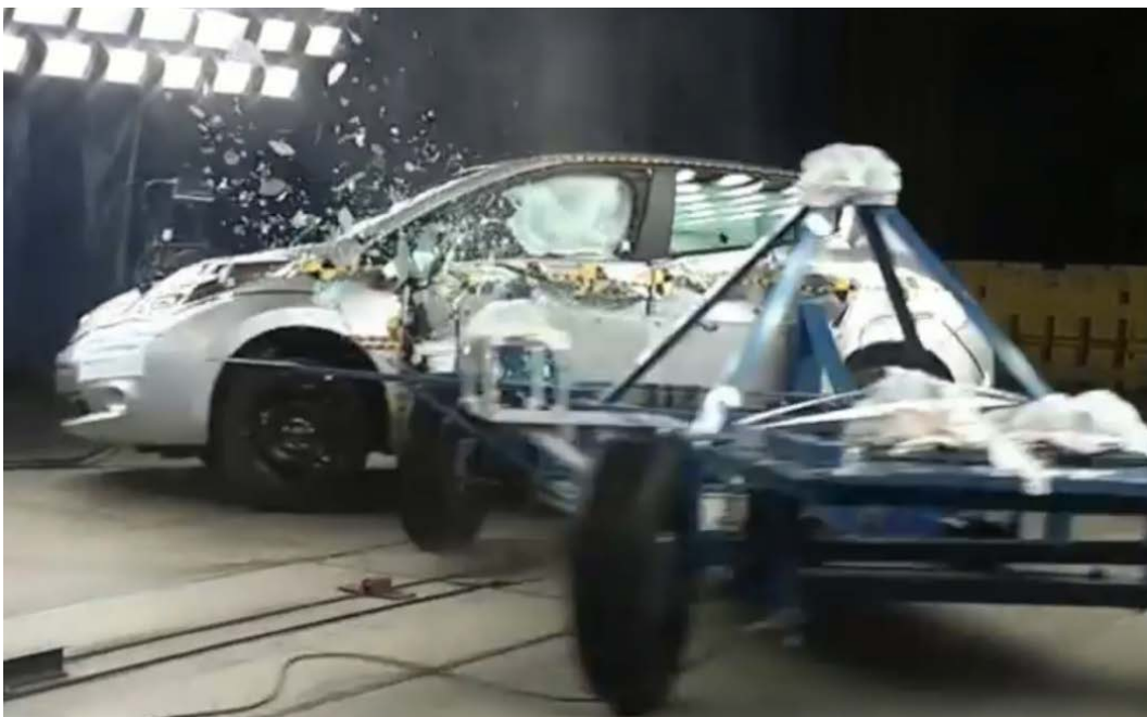
Figur 49 Side Impact Crash – NHTSA NCAP Crash Test Video 2013 Nissan LEAF 5DR Hatchback (92)
