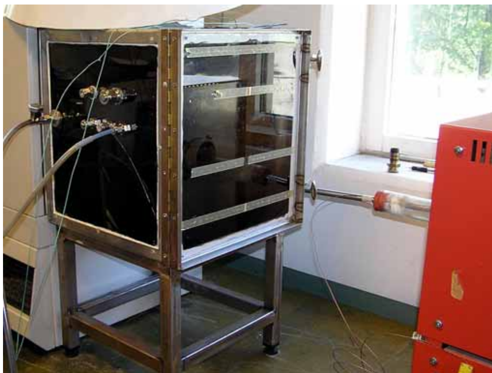
Figure 2 The connection between the mixing chamber of the primary tube furnace (left) and the secondary tube furnace (red coloured to the right).
