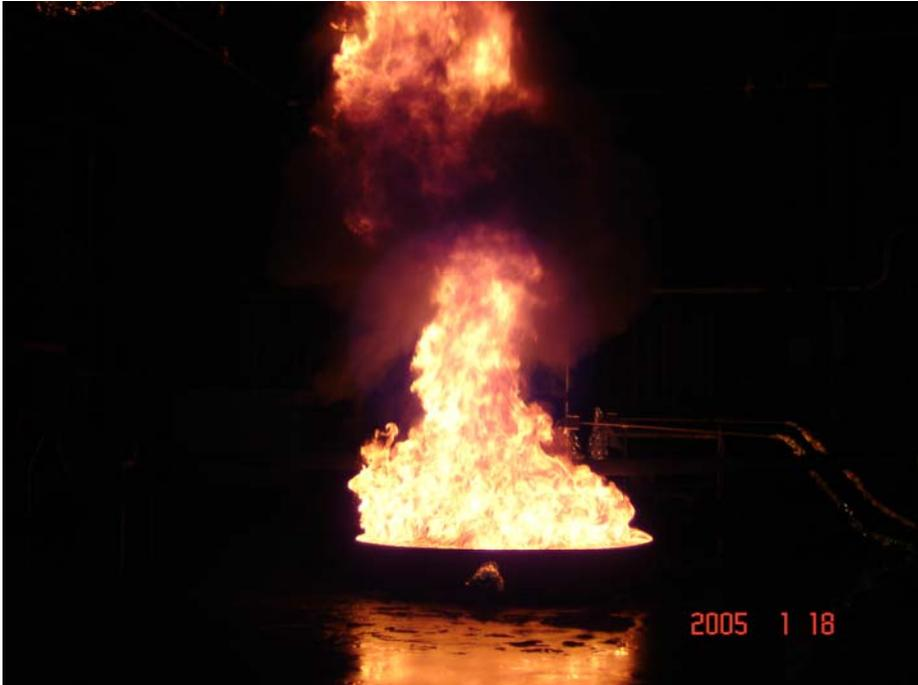
*Photo 1 Free-burn of the 3,5 MW diesel pool fire.*
