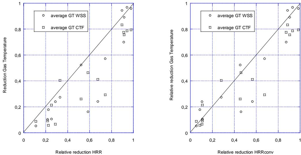
*Figure 10 The relative reduction in average gas temperature versus the relative reduction in the measured  $HRR_{tot}$  (left) and  $HRR_{conv}$  (right) for all the performed tests. The line represents equal values for both axis.*
