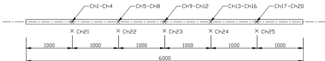
Figure 2 The position of the thermocouples along the length of the Pipe Thermometer.
