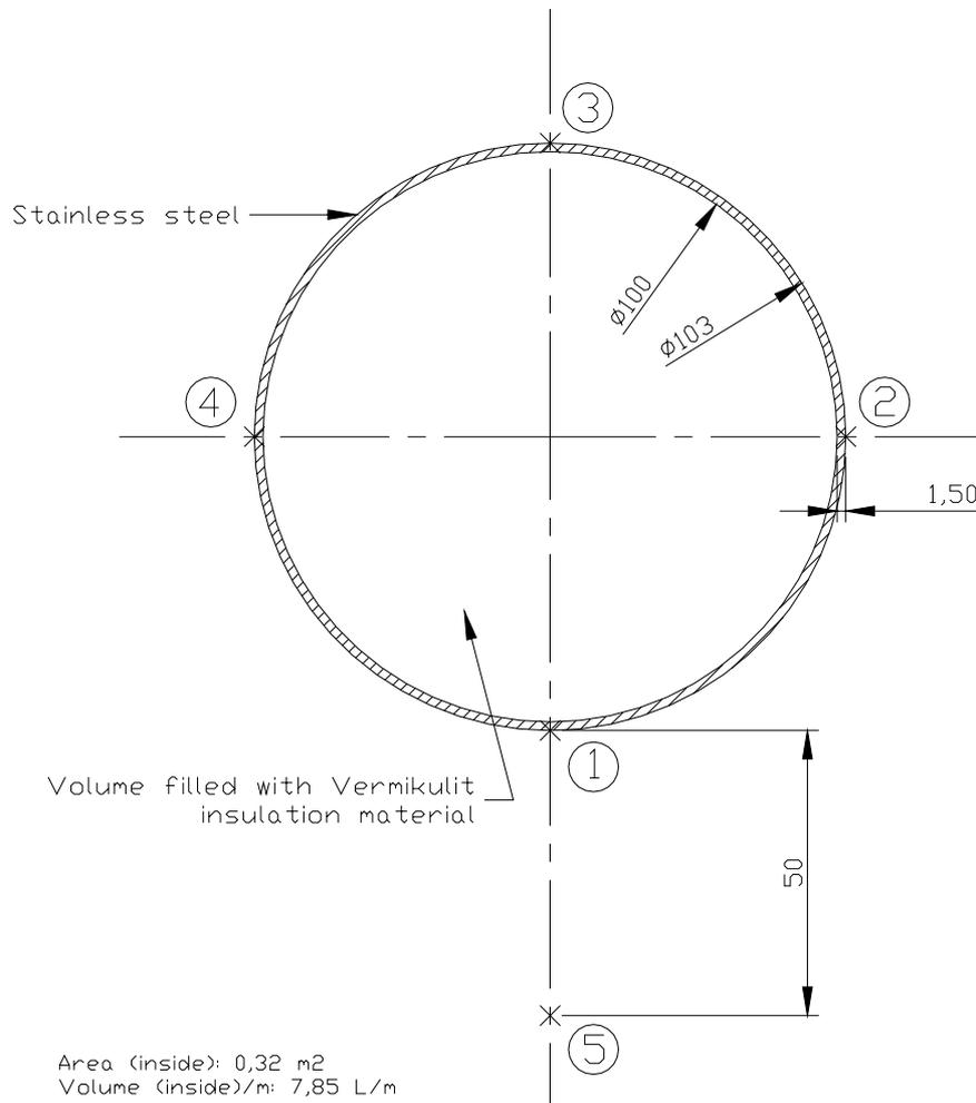
Figure 1 The Pipe Thermometer with the position of the thermocouples on the perimeter of the pipe.
