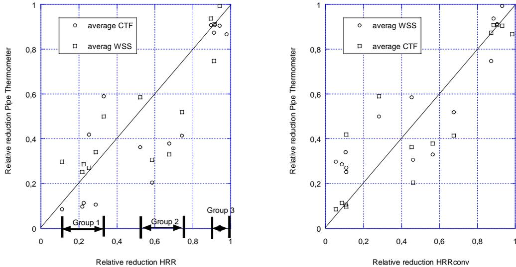
Figure 9 The relative reduction in average surface temperature (1, 3 and 5 points) of the Pipe Thermometer versus the relative reduction in the measured  $HRR_{tot}$  (left) and relative reduction in the  $HRR_{conv}$  (right) for all the performed tests. The line represents equal values for both axis.
