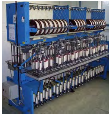
Figure 9: Wick Braiding Machine
