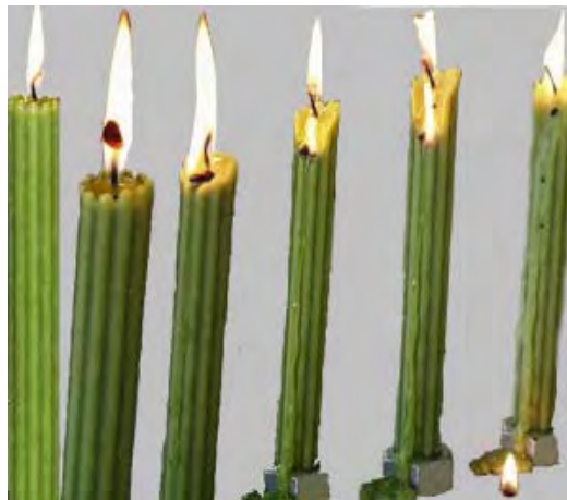
Figure 18: Formation of Second Wicks Caused by Debris Resulting from Mushrooming
