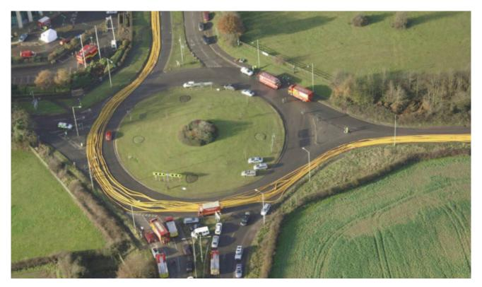
Figure 7 Fire hose expertly laid around the Breakspear roundabout and connecting the fire ground with the water source (the Breakspear lagoon)
