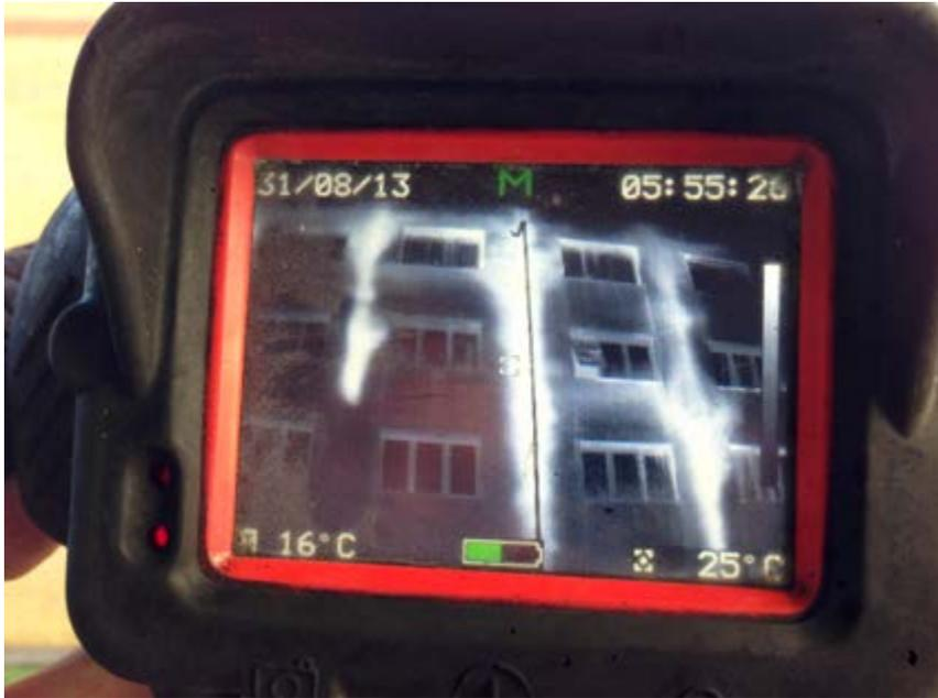
A thermal imaging camera is a valuable tool for finding hidden structural fires, but it can provide incorrect information because the heat conduction through, for example, a wall takes some time. The image shows a modular multi-family building with fire spread between the modules. Photo: Christer Björkman.
