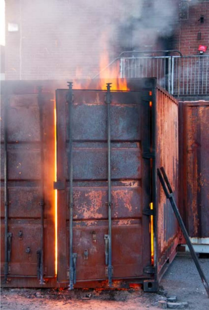
In a steel container, which is often used in fire service exercises, fire spreads in different ways than in a real furnished room, because the thermal inertia of walls and ceiling is different. Photo: Stefan Svensson.
