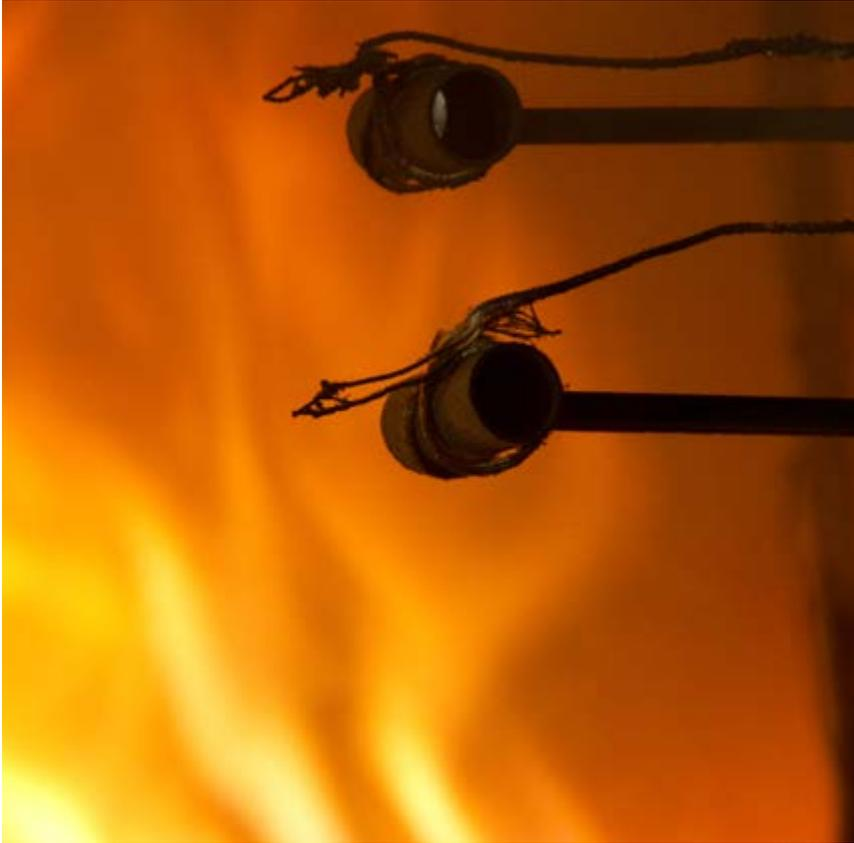
Fire research is often experimental. The image shows two thermocouples (to measure temperature) each mounted on so-called bi-directional probe (to measure and calculate the velocity of gases). Photo: Stefan Svensson.
