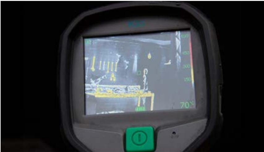
Different materials can have different emissivity and are therefore perceived differently in, for example, a thermal camera. Photo: Stefan Svensson.
