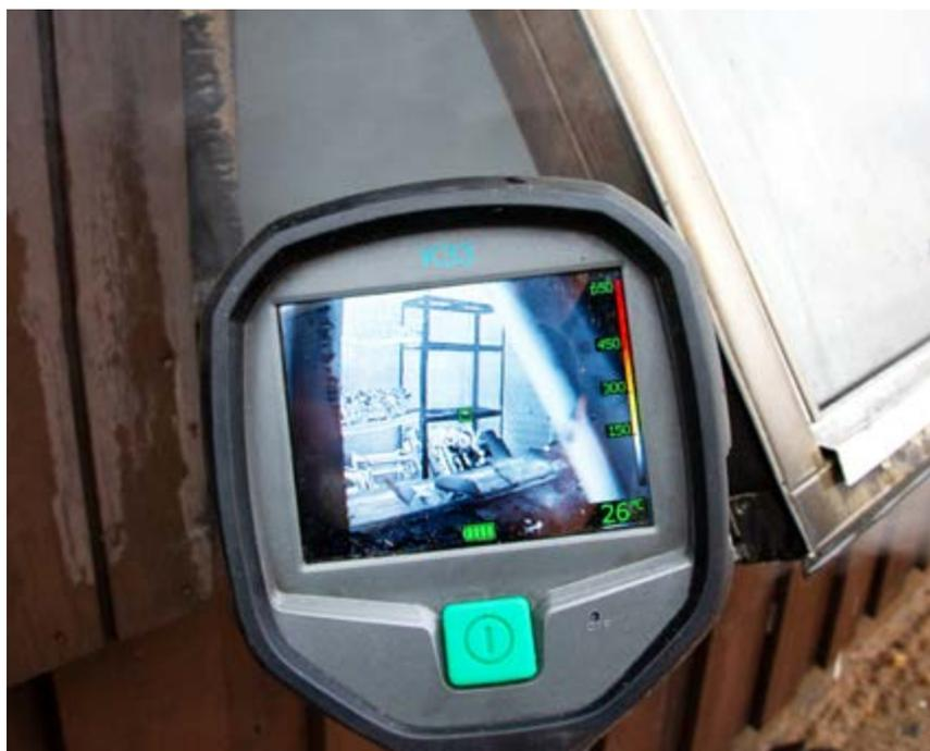
Using an IR camera, we can detect and identify, for example, various objects through fire gases. Photo: Stefan Svensson.
