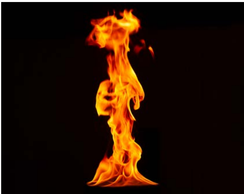
Turbulent diffusionsflamma. Foto: Stefan Svensson.
