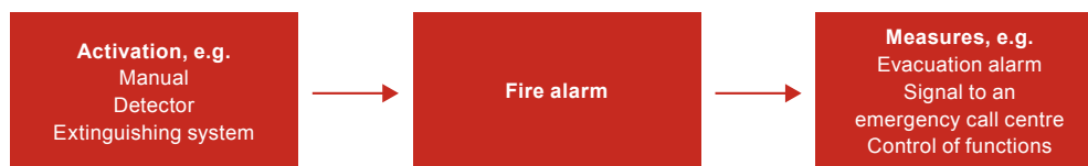
Figure 14. Fire alarm functions
