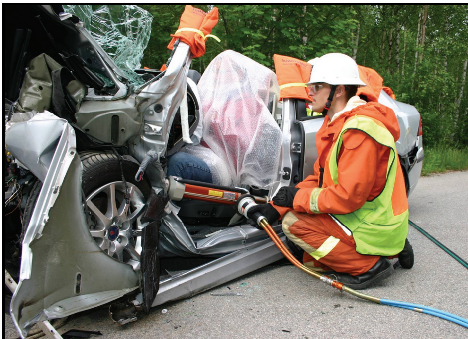
Figure 6. A hydraulic ram can also be applied between the A- and B-posts in order to release the trapped occupant (Photo: SRSA).
