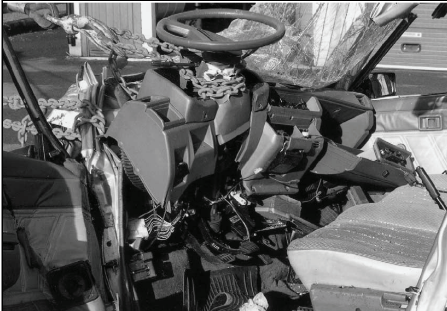
Figure 3. The pull is finished and the space between steering wheel and the dashboard is widened [4].
