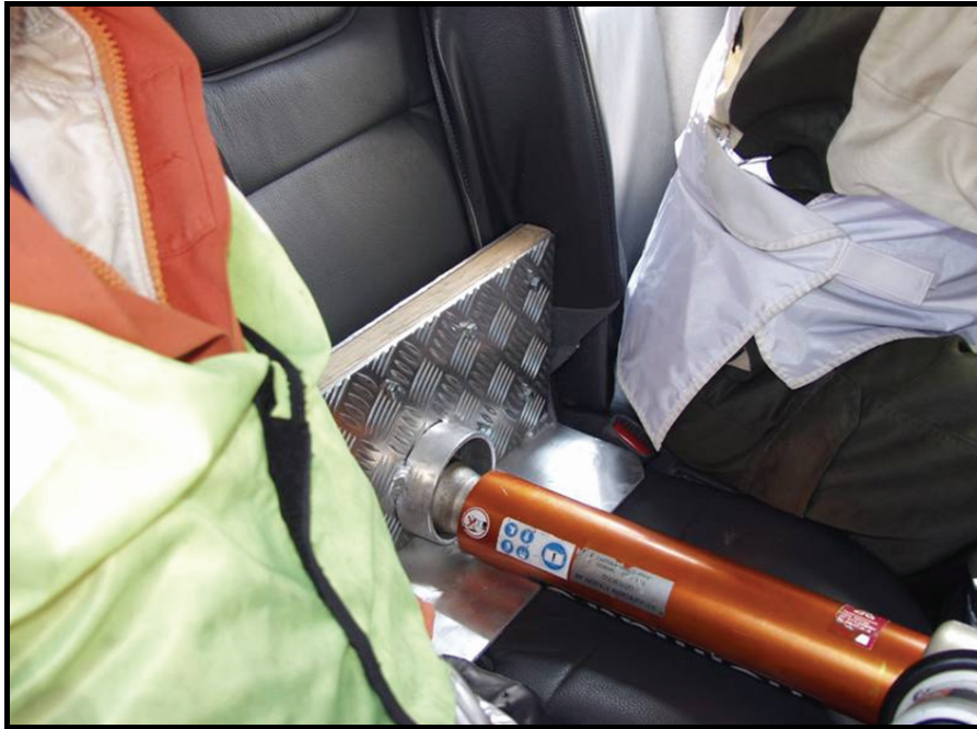
Figure 5. A hydraulic ram pressing the dashboard towards its original position in order to extricate the trapped occupant (Photo: SRSA).
