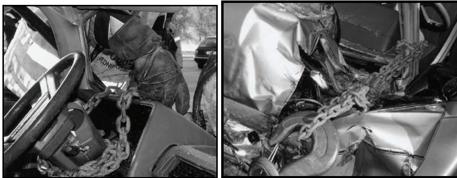
Figure 1. A chain is positioned around the steering wheel and the base of the A-post [4].
