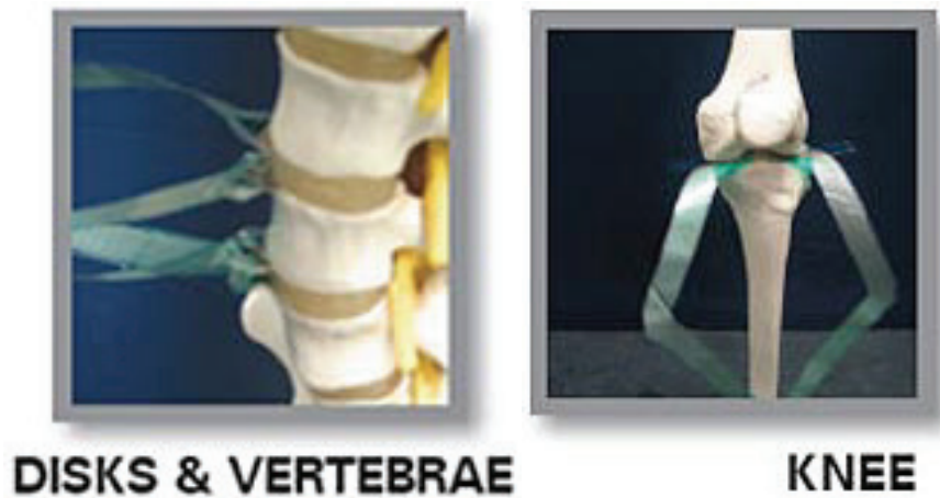
Figure 20. Two examples of how the thin pressure sensor K-scan can be applied, in between vertebrae and in a knee joint.
