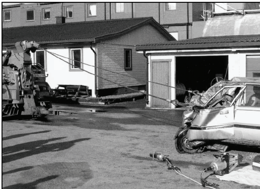
Figure 2. The winch pulls the steering wheel and dashboard away from the front seat via chains and wire [4].
