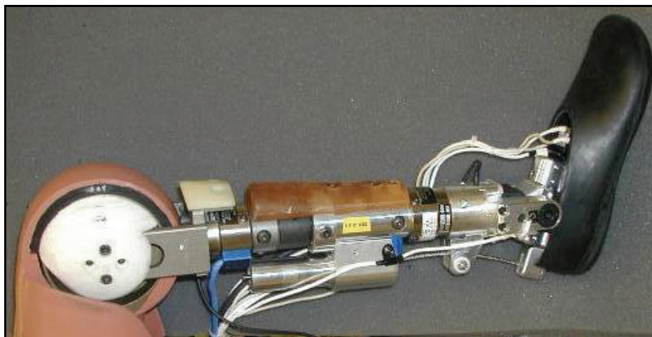
Figure 15 The Thor-Lx leg without artificial skin coating.
