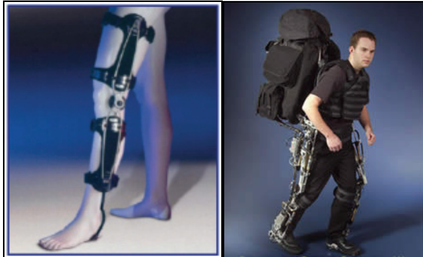
Figure 18. The picture on the left shows an orthosis for knee support developed by Otto Bock Healthcare. The picture on the right shows the wearable exoskeleton BLEEX developed by the Berkely Robotic Laboratory.
