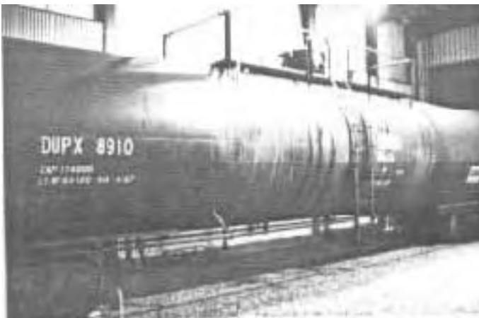
Sodium tank cars are loaded in a dry environment.
