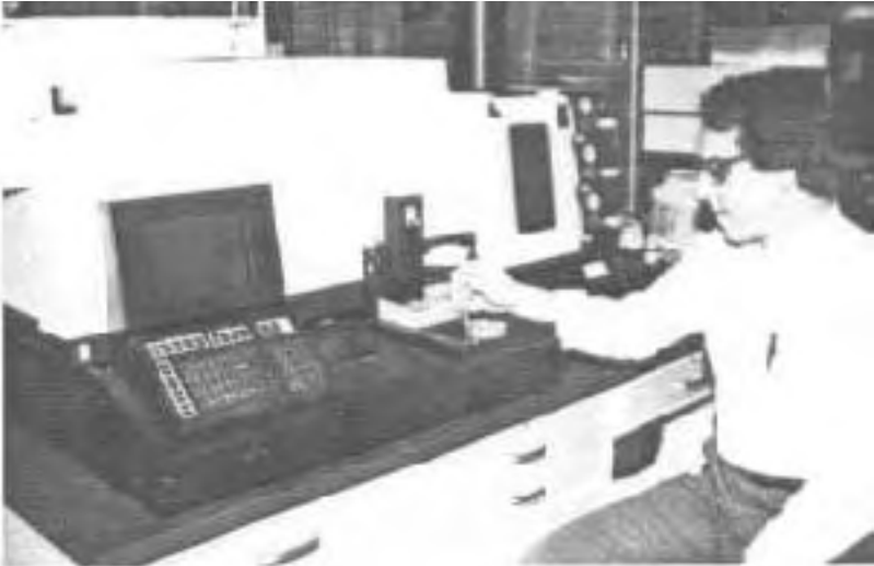
Both direct current and inductively coupled plasma spectrophotometers allow trace impurity analyses for product and raw materials.
