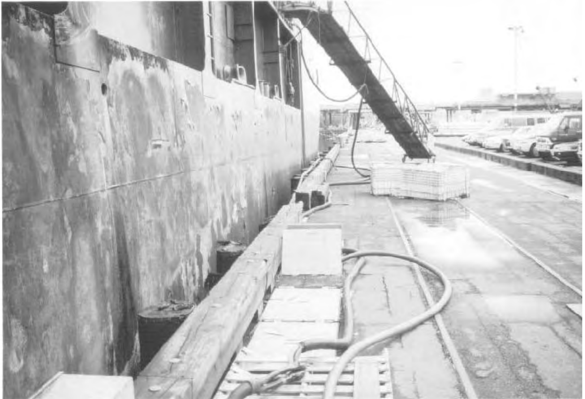
Port side - maximum discoloration near Hold #3; paint in good condition toward bow; note that the hull did not buckle.
