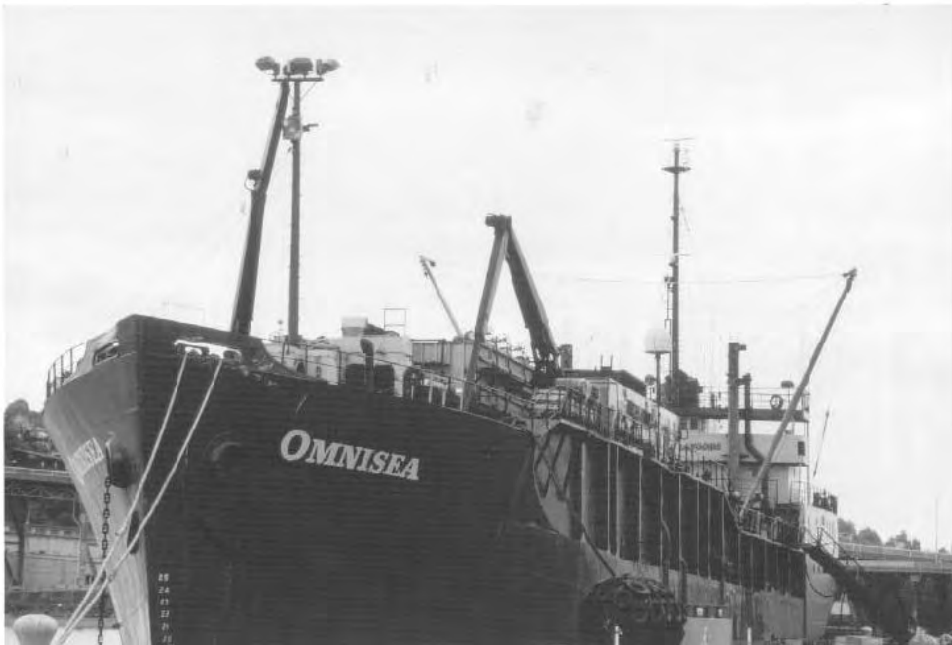
Bow of Omnisea . Note amount of compartments and equipment on deck - a complex area for fire fighting. (Photo by Philip Schaenman)
