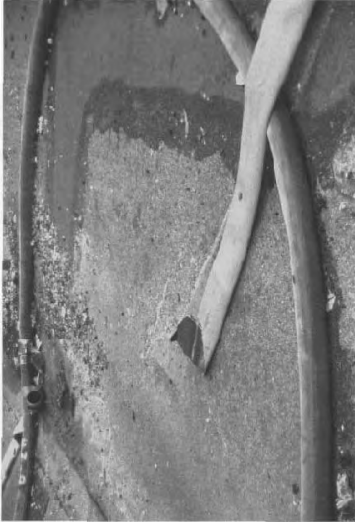
Section of 5-inch hose that was ruptured by falling debris outside the building. Hose lines feeding the standpipes and entering the stairways were damaged several times and had to be replaced at great risk to firefighters.
