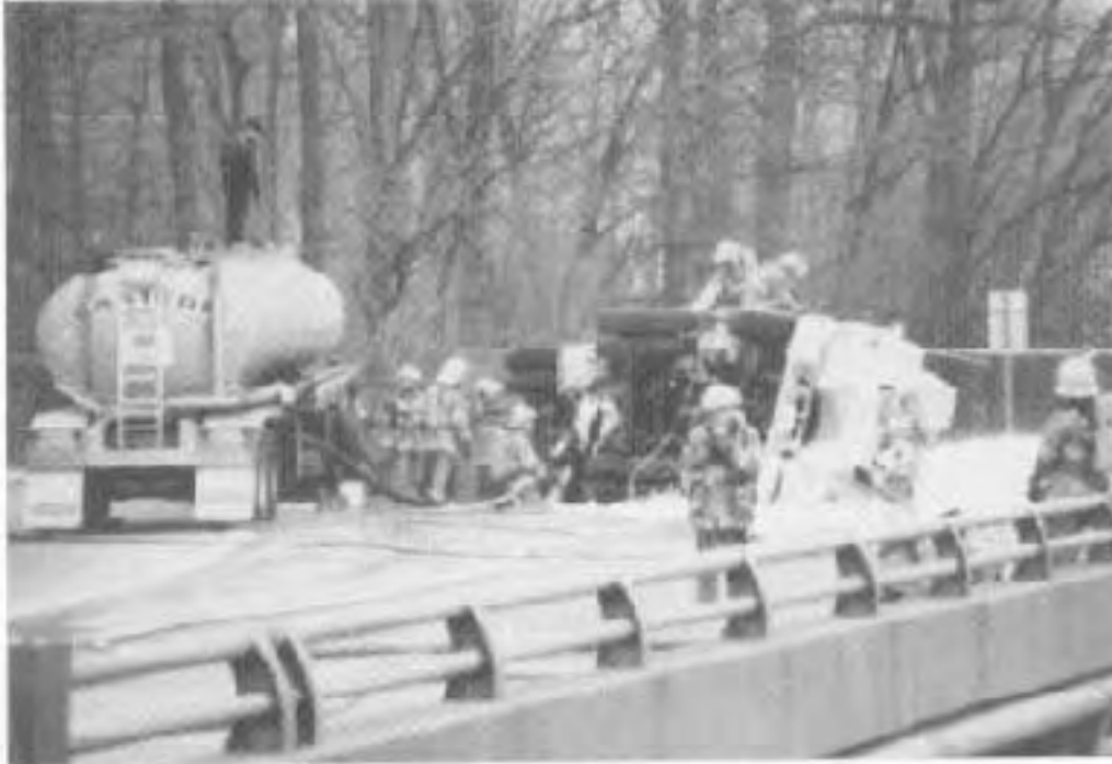
4. Second tanker pumping fuel from the overturned tanker.
