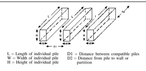
Diagram 3. Cutoff Storage for Class 2 and Class 3 Oxidizers (All distances in feet)
