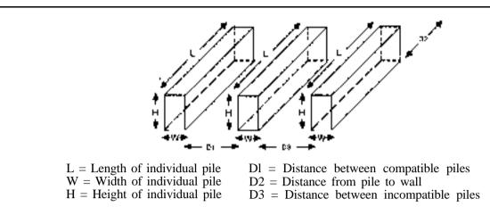
Diagram 1. General Arrangement for Class 1 Oxidizers or Segregated Storage for Class 2 and Class 3 Oxidizers (All distances in feet)
