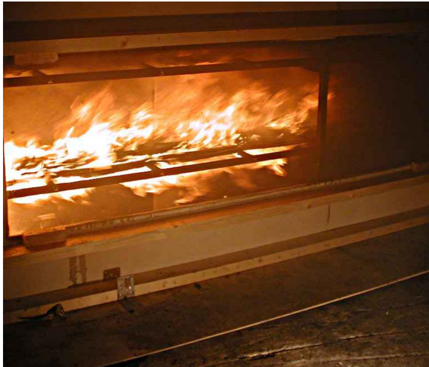
Figure 7. Side view of test H6, forced ventilation rate 3-3.2 m/s. The flames are not reaching the top ladder.
