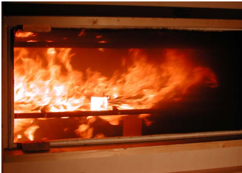
Figure 6. Side view of test H4, forced ventilation rate 1.5-1.8 m/s.
