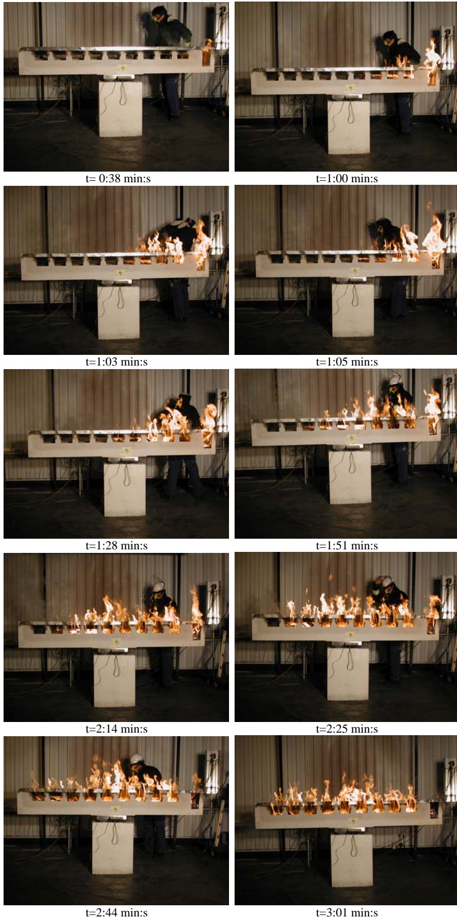
Figure 9 The fire development in test 4 with corrugated cardboard.
