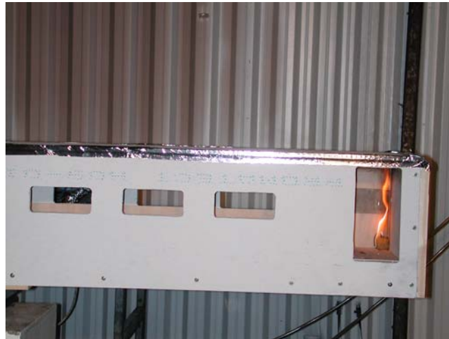
Figure 6 The ignition source consisted of a fibreboard cube soaked in 15 mL heptane which was placed in the corner at floor level.
