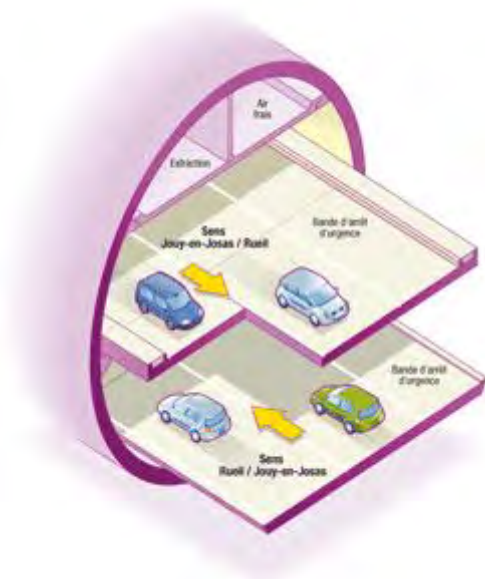
Figure 4 Tunnel section for A86 east link.
