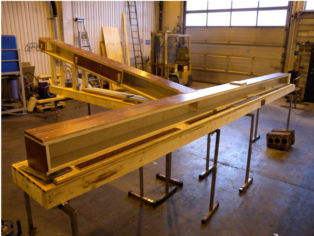
Figure 15 The model-scale tunnel system before the walls and windows were completed.
