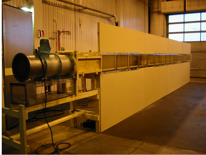
Figure 1 A photo of the 1:23 model scale tunnel before it was used for fire tests with longitudinal ventilation [39]. A fan was attached to the tunnel entrance and windows were put on one side.
